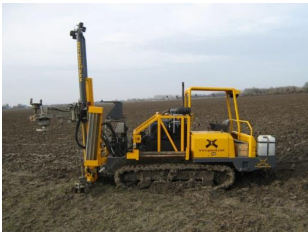
Figure 3.2: A cone penetration test
