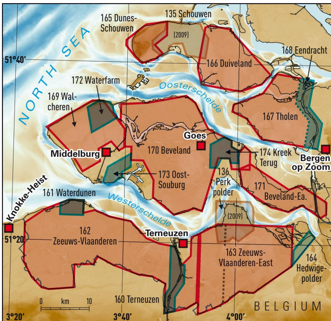
Figure 5.5: Sketch of the airborne survey areas in Zeeland. Areas in green, ochre and red were flown at 100 m, 200 m and 300 m line spacing, respectively. The area Dunes Schouwen was partially flown at 200 m line spacing and 200 m tie-line spacing. The area Oost Souburg was flown at 300 m line spacing.
