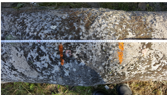
Figure A-3: Photos of diameter changes in pile 8.
