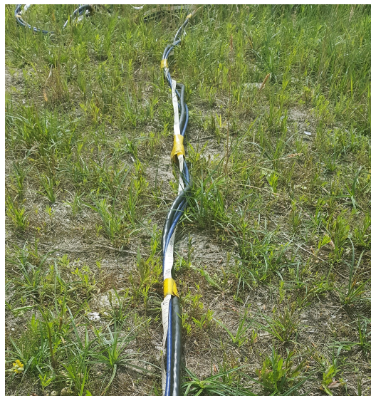
Figure 7-4: Photo of the cable of the Seismic Tube with the measuring tape attached
