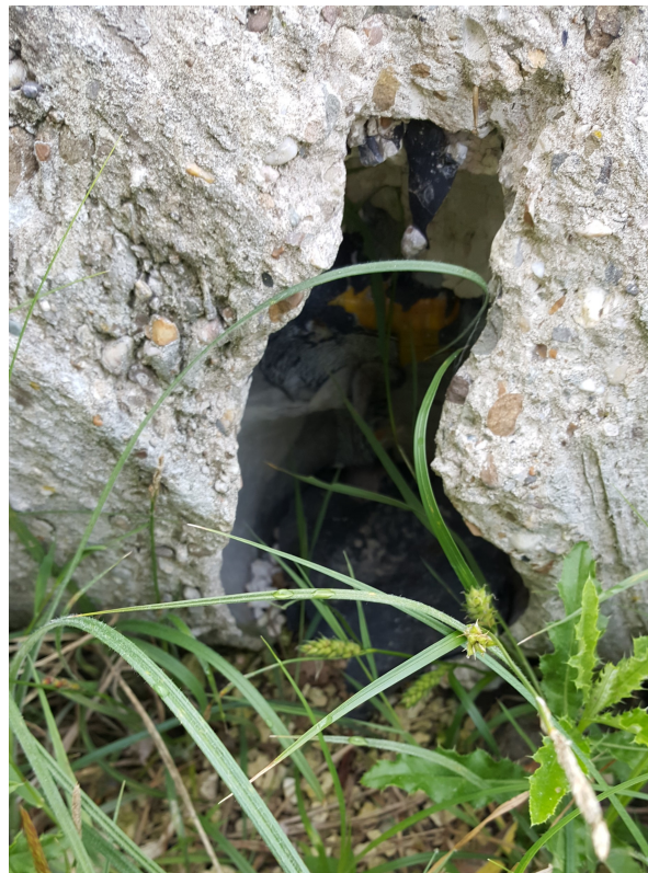
Figure 2-10: Photo of designed neck in test pile 13 at Deltares test site
