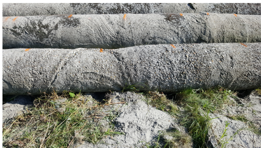
Figure 7-7: Photo of some holes dug underneath the pile to measure the circumference.
