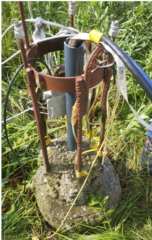
Figure 7-1: Photo of top of Pile 10 the test site at Deltares Delft. The Seismic Tube is lowered in the PVC pipe
