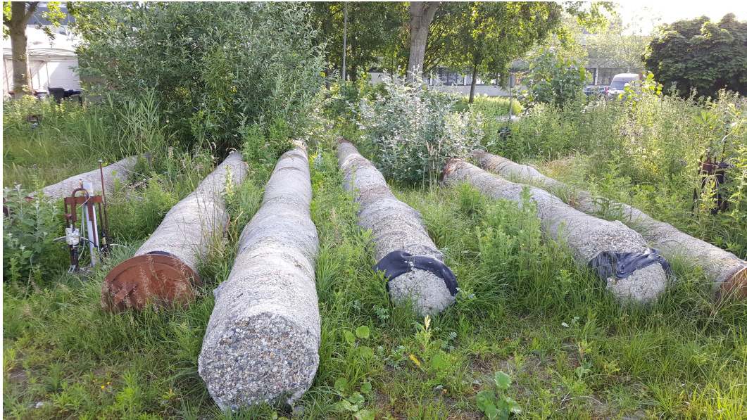
Figure 2-9: Photo of the piles pulled out the ground at Deltares test site. Pile number from left to right: 13, 7, 1, 8, 6, 17.
