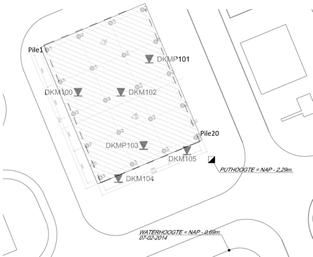
Figure G-1: Location CPT's performed at Deltares test site.
