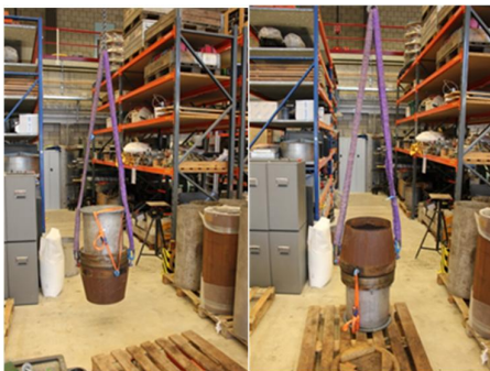
Figure 7. Lifting and rotating of the sampler
