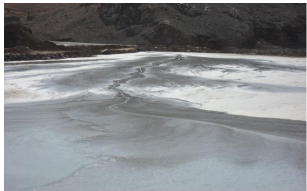
Figure 3. Fines dominated thick tailings beach, with long single channel and expanding flow. Source: B. Pirouz, ATC Williams, Australia.
