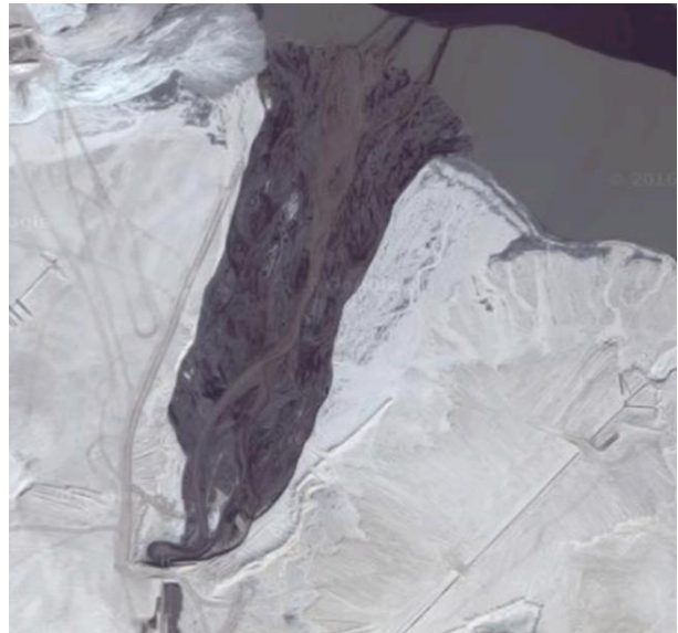
Figure 2. Sand dominated diluted tailings stream from oil sands external facility. Source: Google maps.
