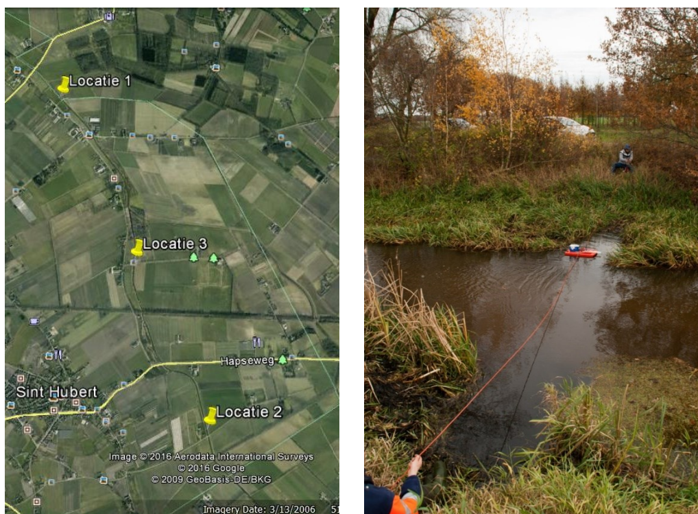
Figure 3.4. Locations at the Lage Raam (left) and ADCP flow measurements at location 3 (right).
