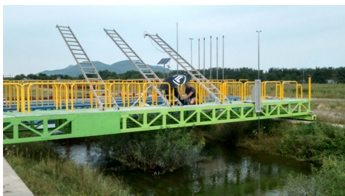
Figure 3.2. The REC experimental set up with a. camera on fixed ladders, and b. on the UAV
