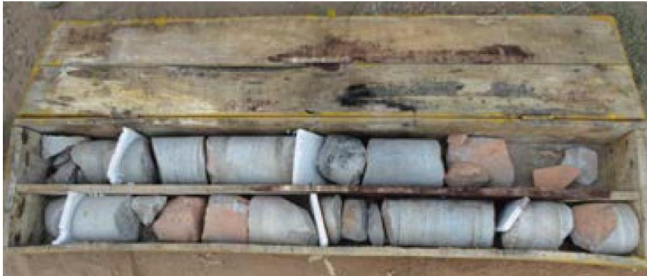
Figure 4.10. Core samples at main dam. Source: CSV20170921.
