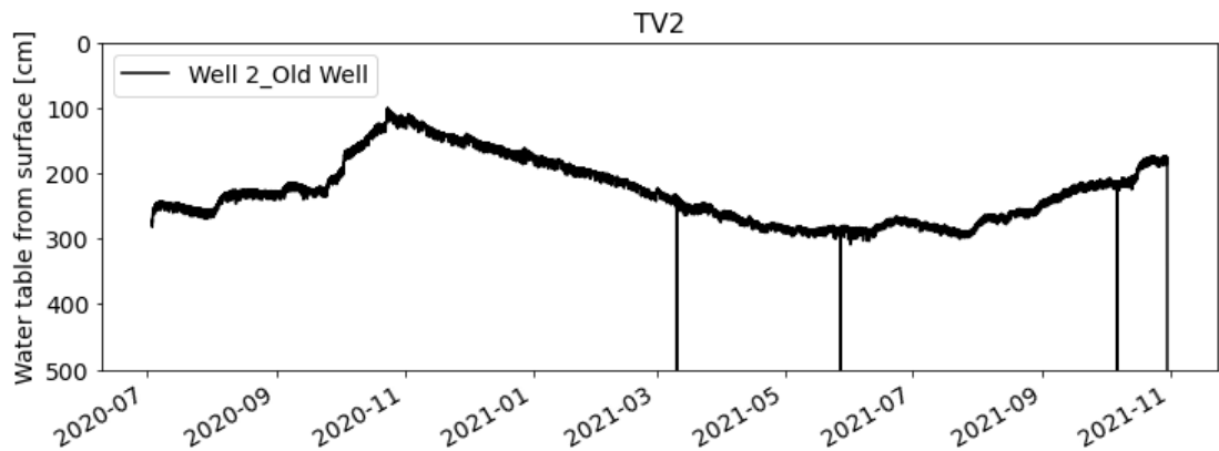
Figure 8-11: The water table depth relative to the surface in TV2 site, recorded in well 2.
