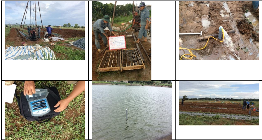
Figure 8-29: Set up the monitoring wells plot with both groundwater and quality (EC).
