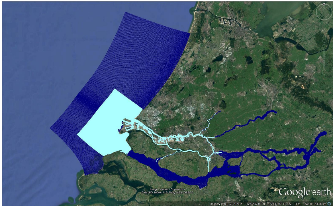
Figure 4-1 Overview of the domains from the OSR model. In dark blue the large domain (Harbour model) and in light blue the smaller domain (NSC).
