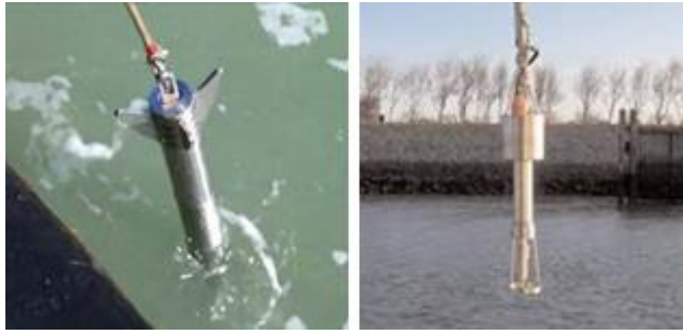
Figure 1-7 Left: the Graviprobe. Right: the Rheotune
