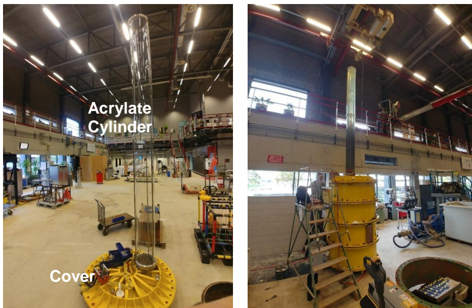
Figure 3-2: Container cover with additional acrylate cylinder.
