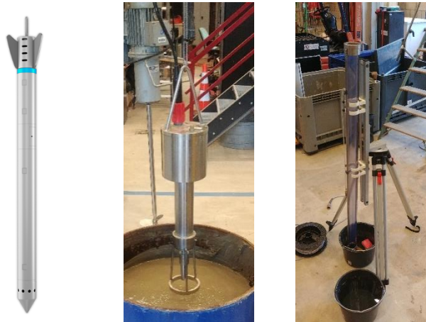
Figure B1: Overview of the used tools. From left to right: the GraviProbe, RheoTune and Beaker Sampler.
