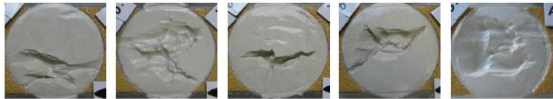
Figure A.3.3 Examples of eroded surfaces with cracks (Jacobs 2011)
