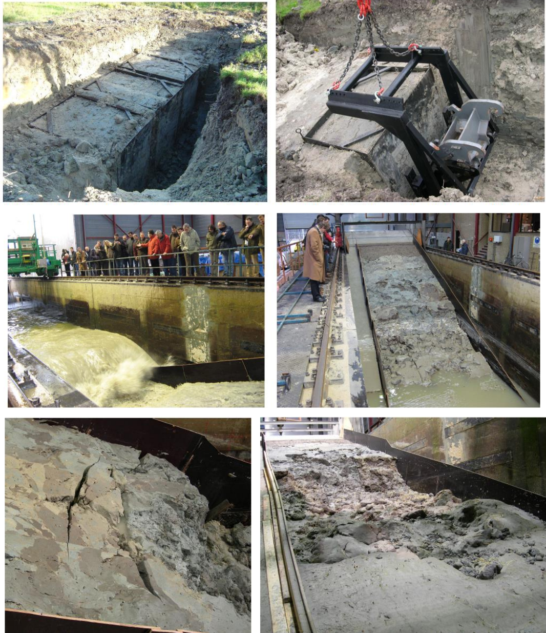
Figure B.2.3 Dutch boulder clay (upper: excavation at local dike; lower: tests in Delta flume)
