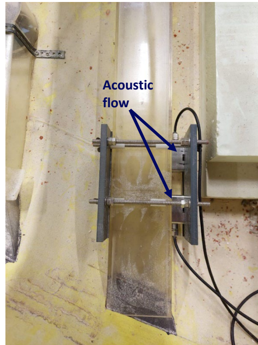
Figure 4.5 The acoustic flowmeter (consisting of the two metal transducers) attached to the bow thruster channel. They are clamped to the Perspex channel by the means of a grey PVC clamp.
