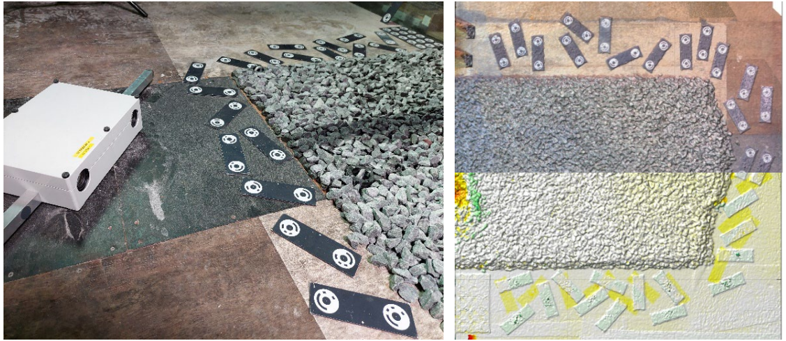
Figure 4.3 Left: The stereophotography setup with on the left the stereo box used to take the images. The region of interest is surrounded by markers to calibrate the images. Right: Example of stereophotography measurement of a loose rock test: bathymetry difference plot on the lower side showing bathymetry changes relative to the initial rock protection level and colour image on the top side, also obtained with stereophotography.
