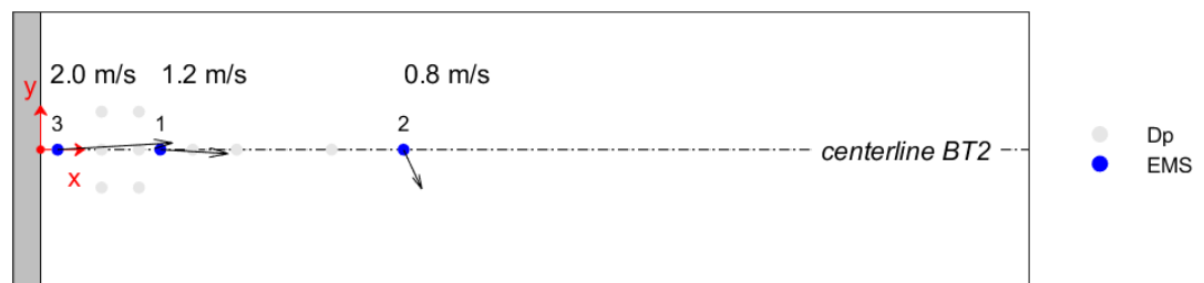
Figure 7.3 Time-averaged flow velocity near the bed measured by the EMS sensors in test 300 (a repetition of test 107). See Figure 3.6 for the exact location of the sensors.
