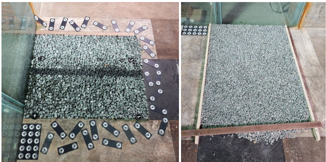
Figure 3.16 Rock gradings used during the rough bed tests. Left: fixed rock 10-60 kg, right: loose rock 90-250 mm.
