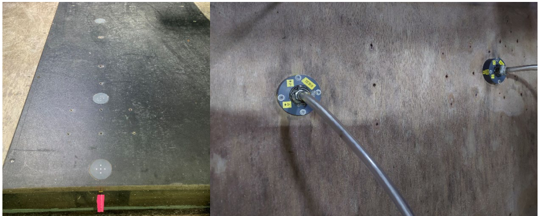
Figure 4.7 Left: Three electromagnetic flow meters mounted flush in the smooth bed. Right: Flow meters seen from the bottom of the bed.
