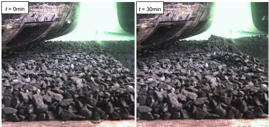
Figure 7.47 Snapshots from Cam1 at the start and end of the test with UKC = 0.5 m. Time in model scale.
