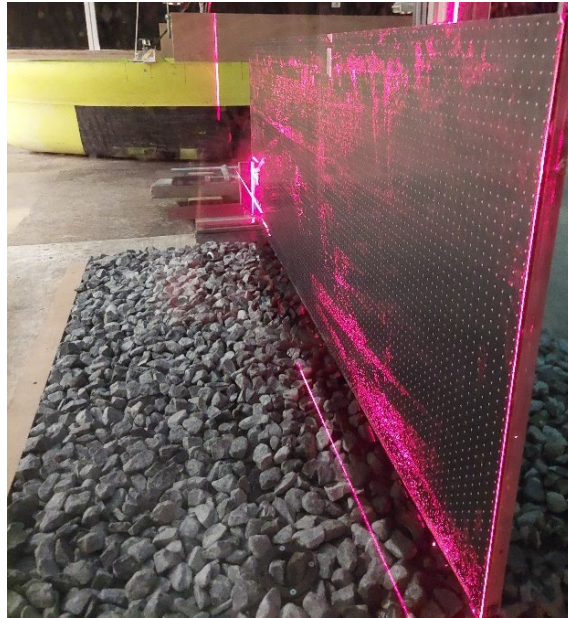
Figure 4.2 The calibration plate aligned with the PIV measurement plane with the aid of a building laser.
