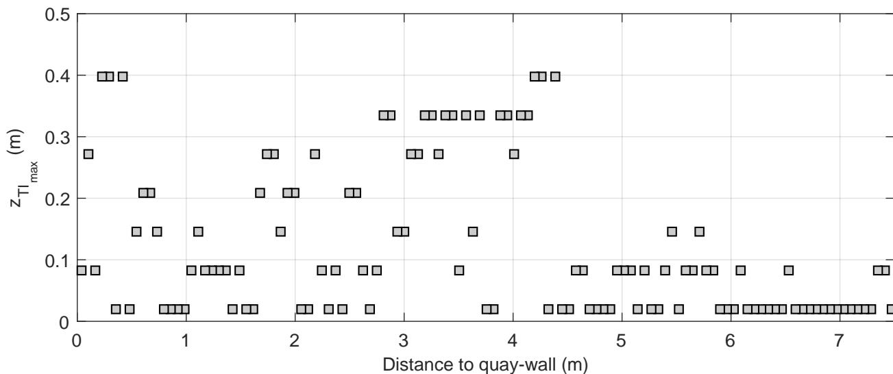
Turbulence intensity profiles | Active thruster: BT2
