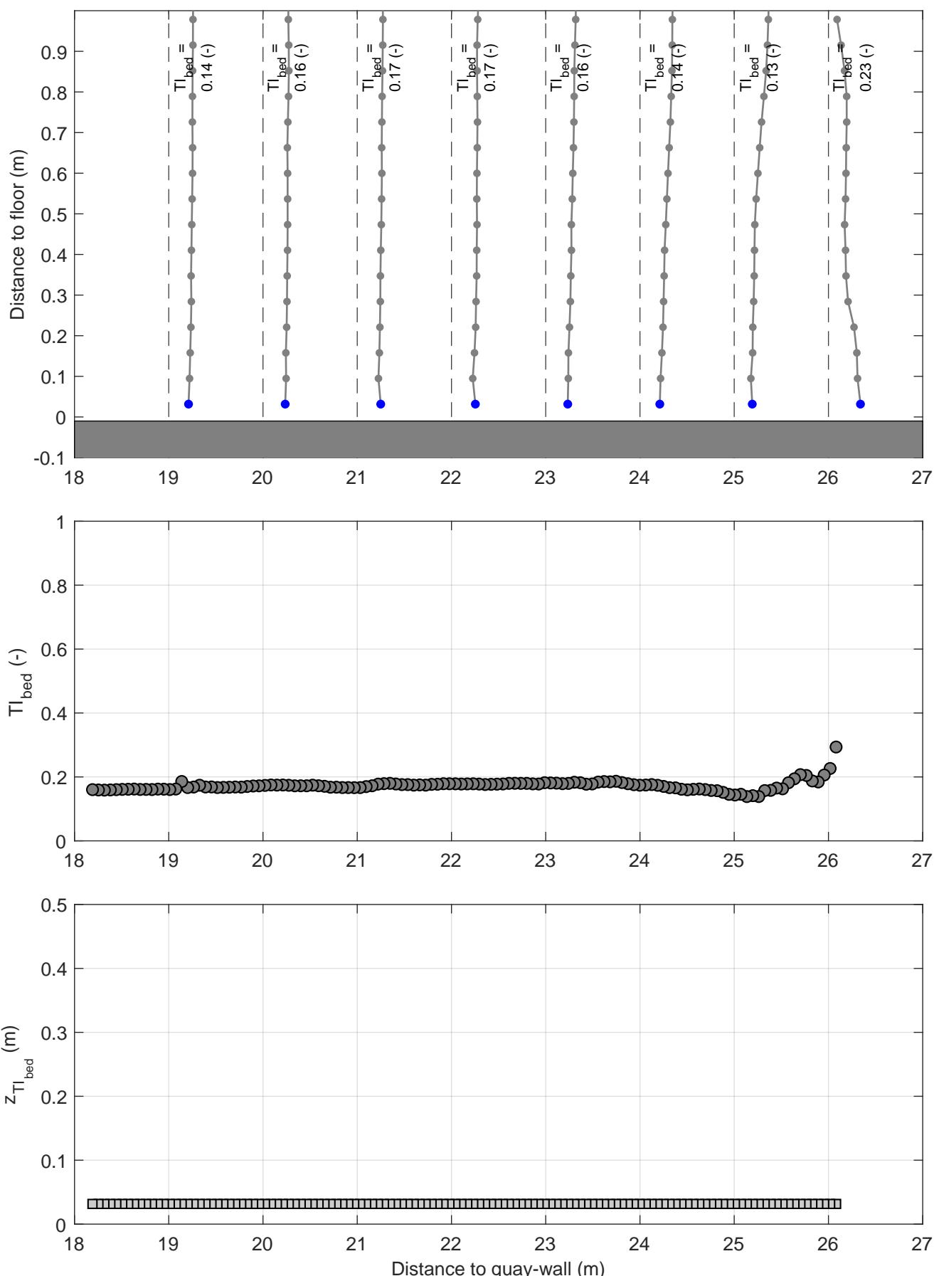
Turbulence intensity profiles | Active thruster: BT1&BT2
