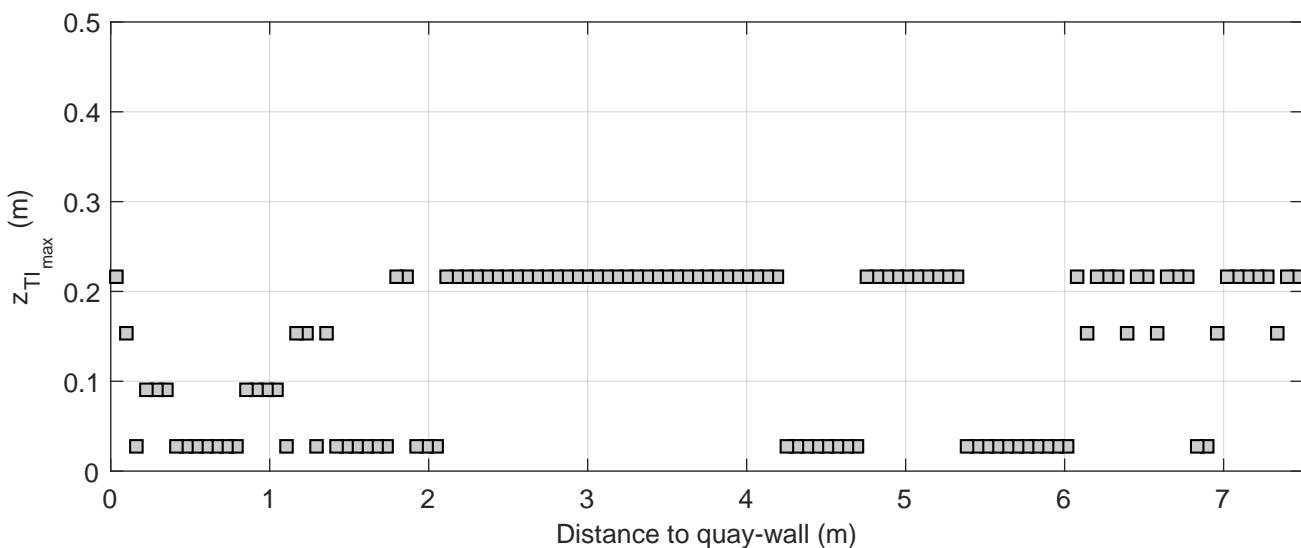
Turbulence intensity profiles | Active thruster: BT1&BT2
