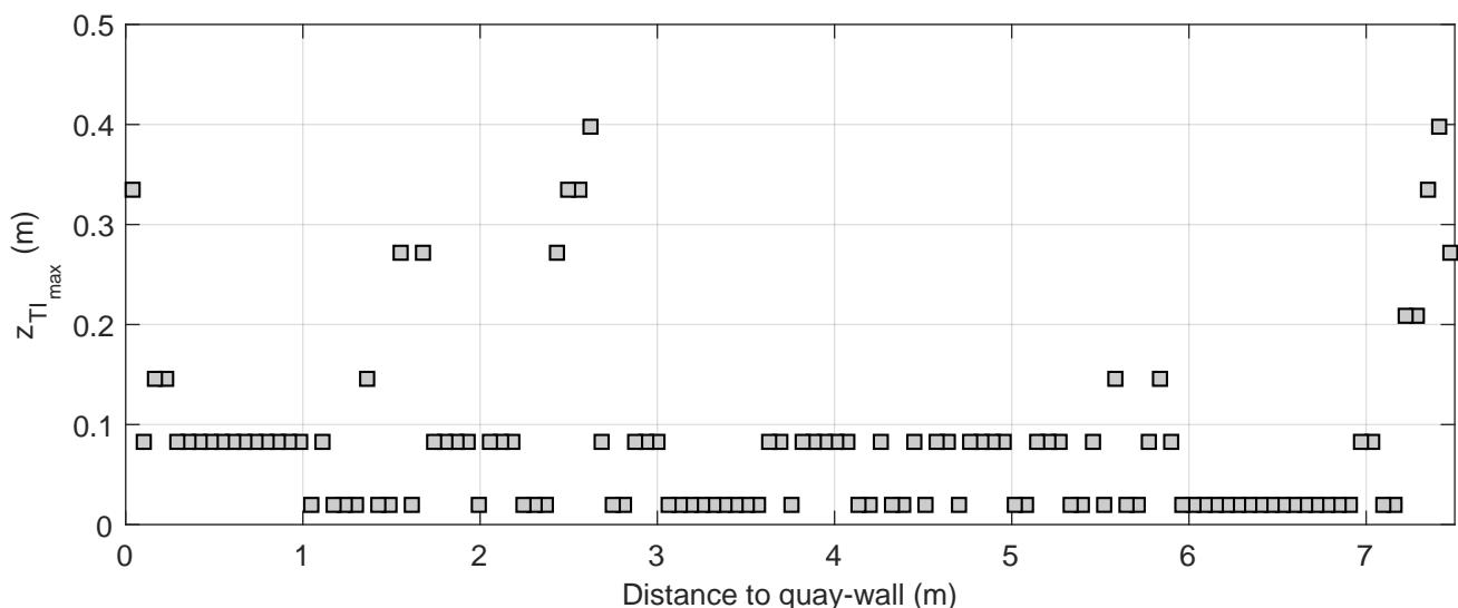
Turbulence intensity profiles | Active thruster: BT2
