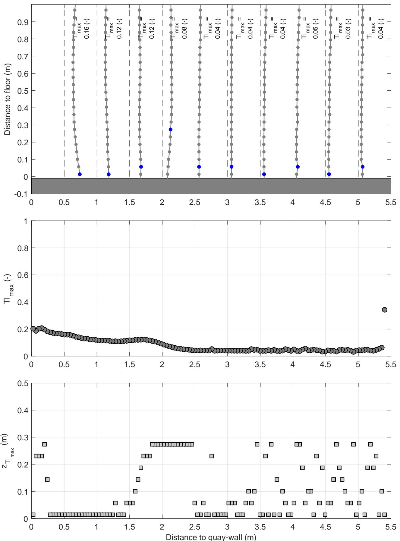
Turbulence intensity profiles | Active thruster: BT2
