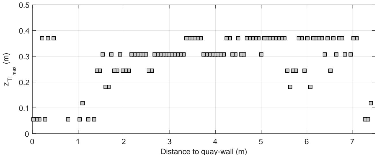
Turbulence intensity profiles | Active thruster: BT2
