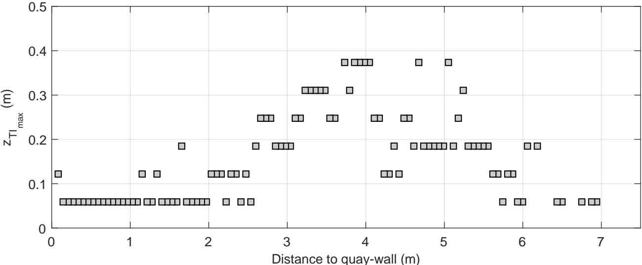
Turbulence intensity profiles | Active thruster: BT2
