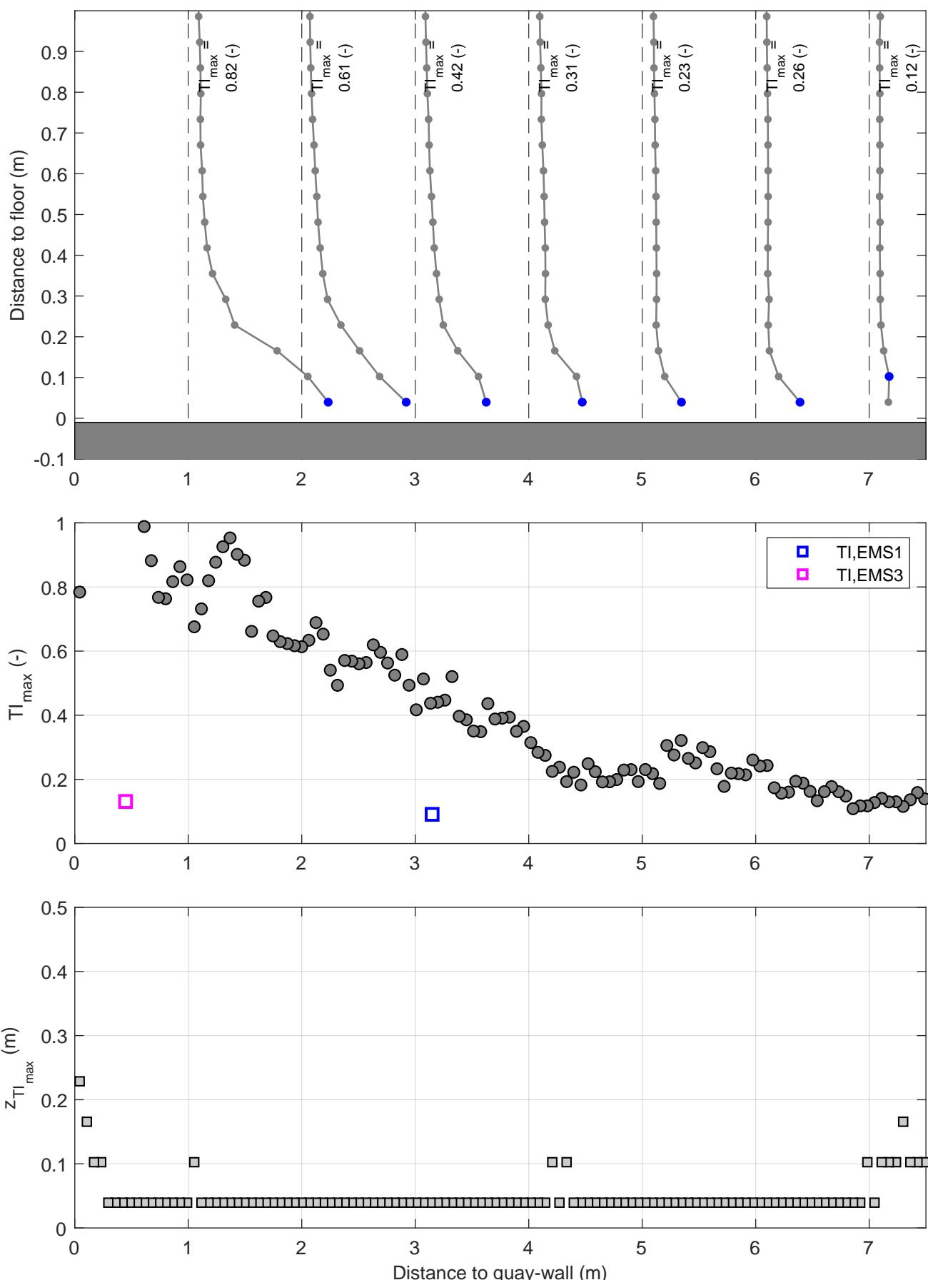
Turbulence intensity profiles | Active thruster: BT1
