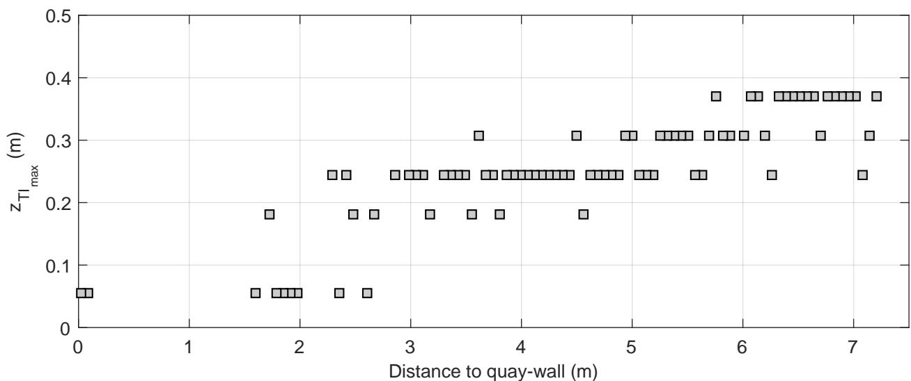
Turbulence intensity profiles | Active thruster: BT2
