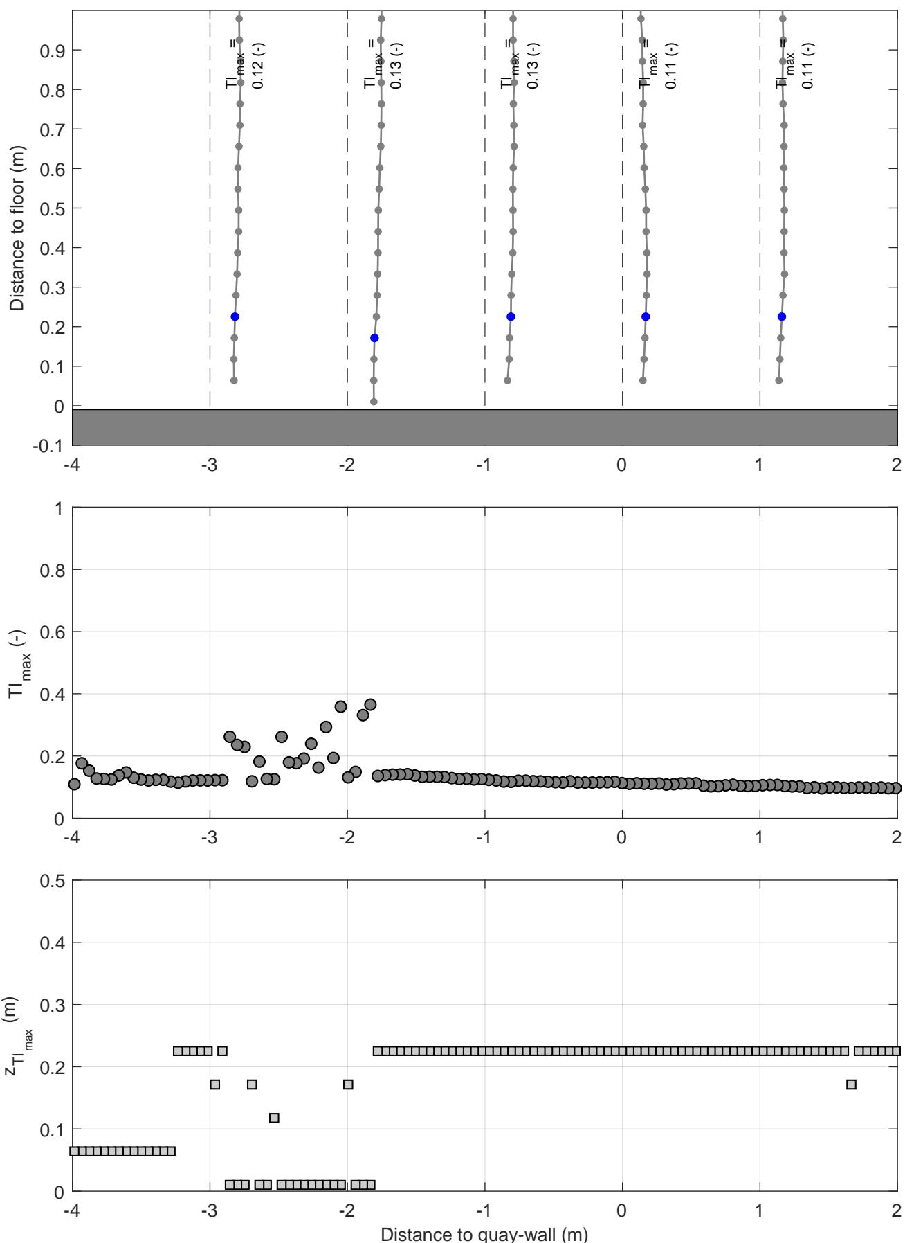
Turbulence intensity profiles | Active thruster: BT2
