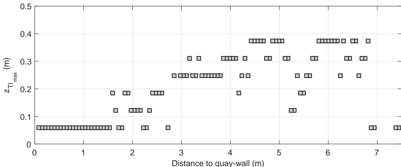
Turbulence intensity profiles | Active thruster: BT2
