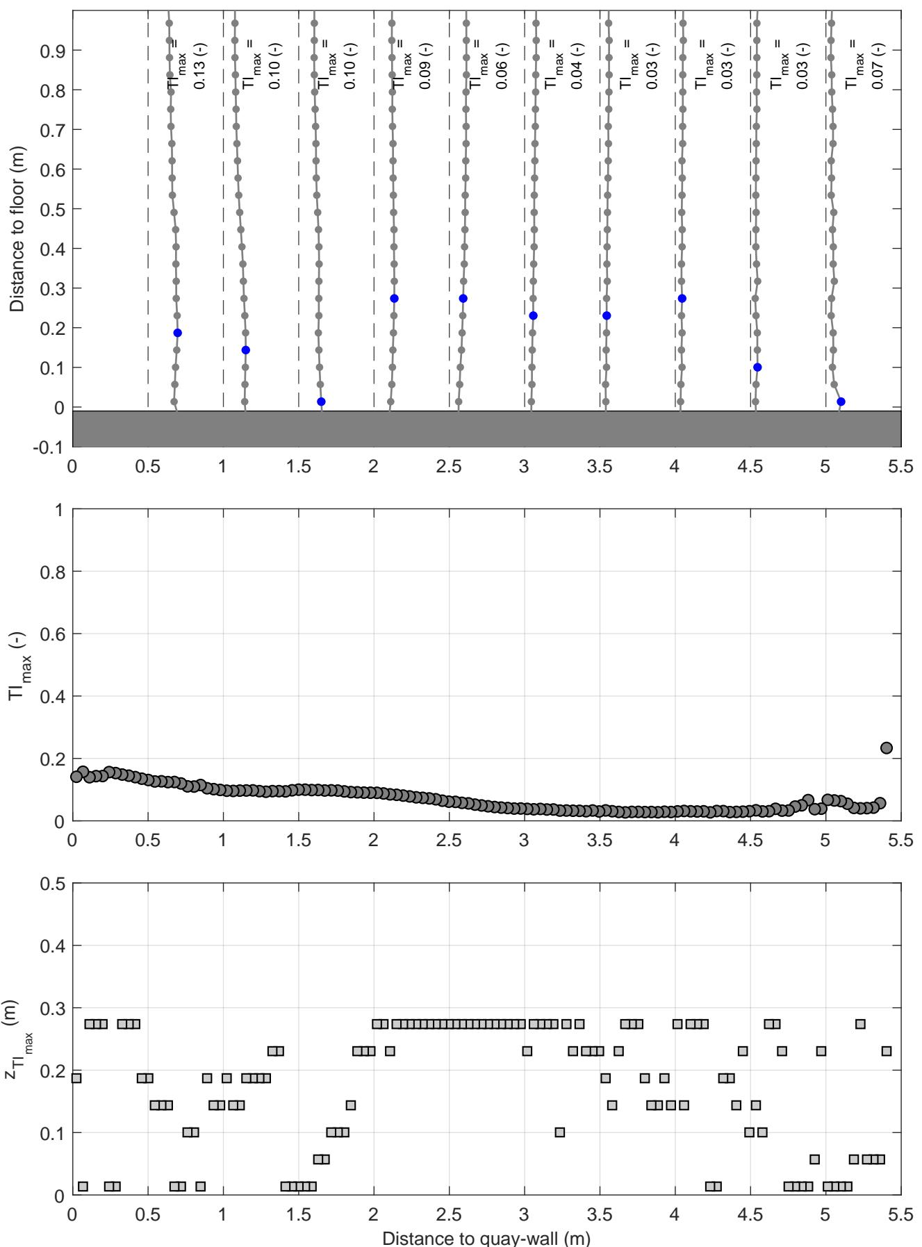
Turbulence intensity profiles | Active thruster: BT2
