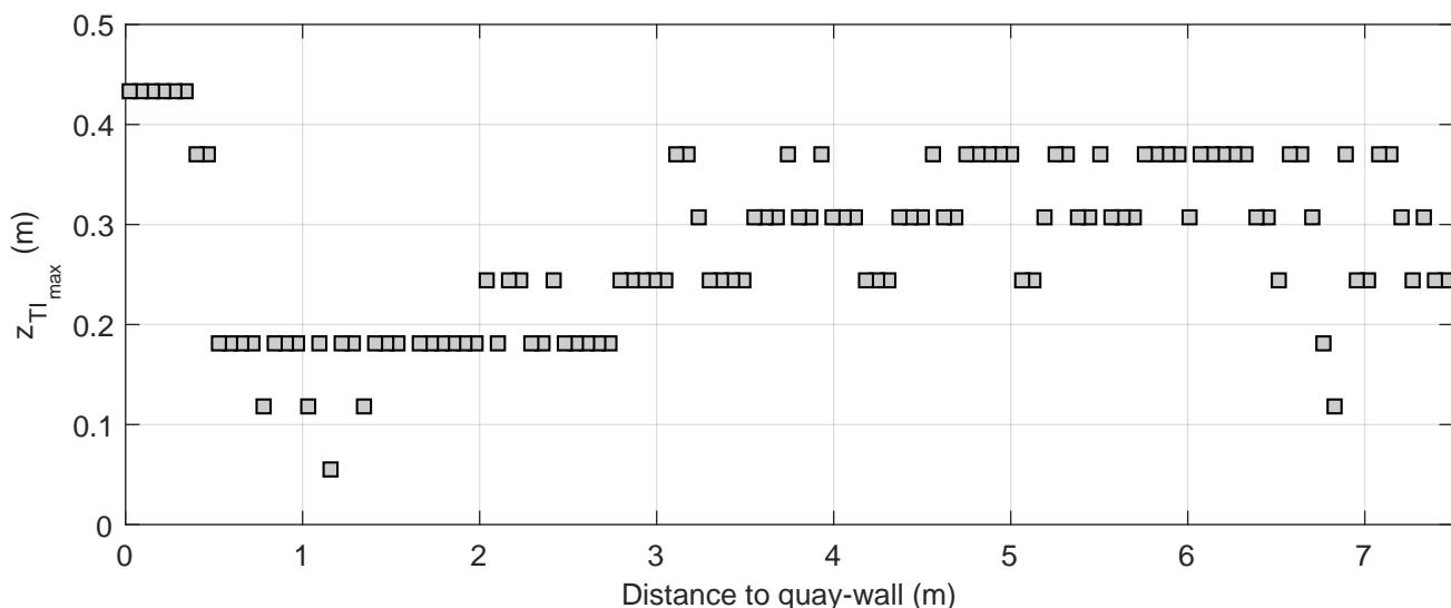
Turbulence intensity profiles | Active thruster: BT2
