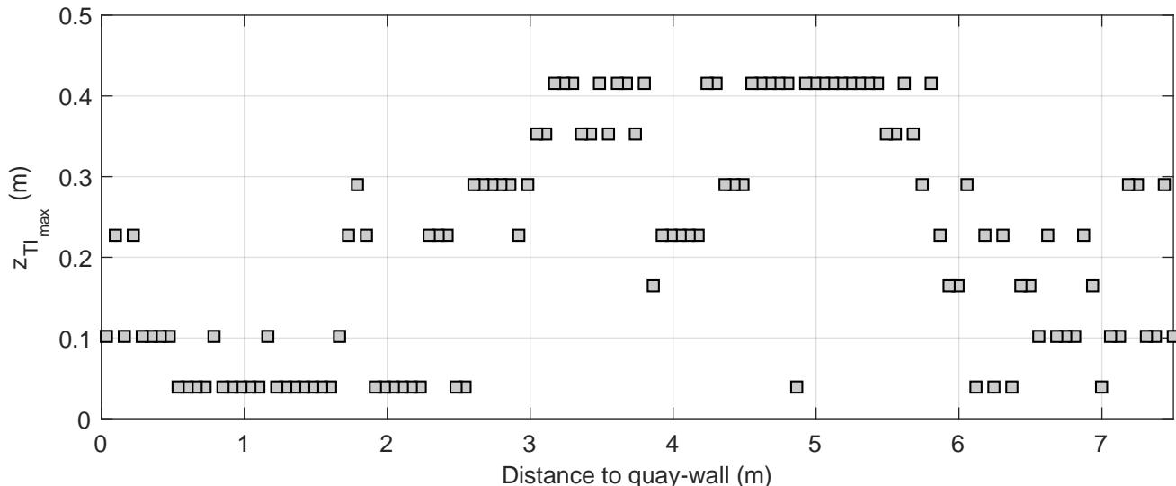
Turbulence intensity profiles | Active thruster: BT1&BT2
