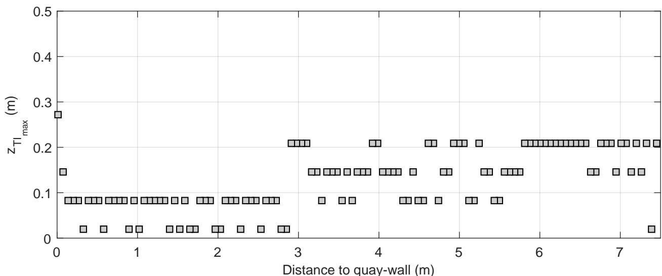
Turbulence intensity profiles | Active thruster: BT2
