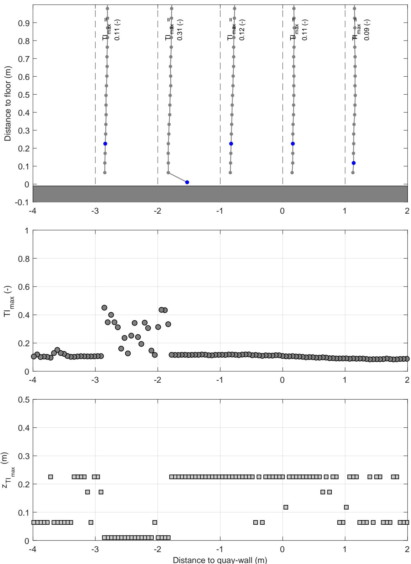
Turbulence intensity profiles | Active thruster: BT2
