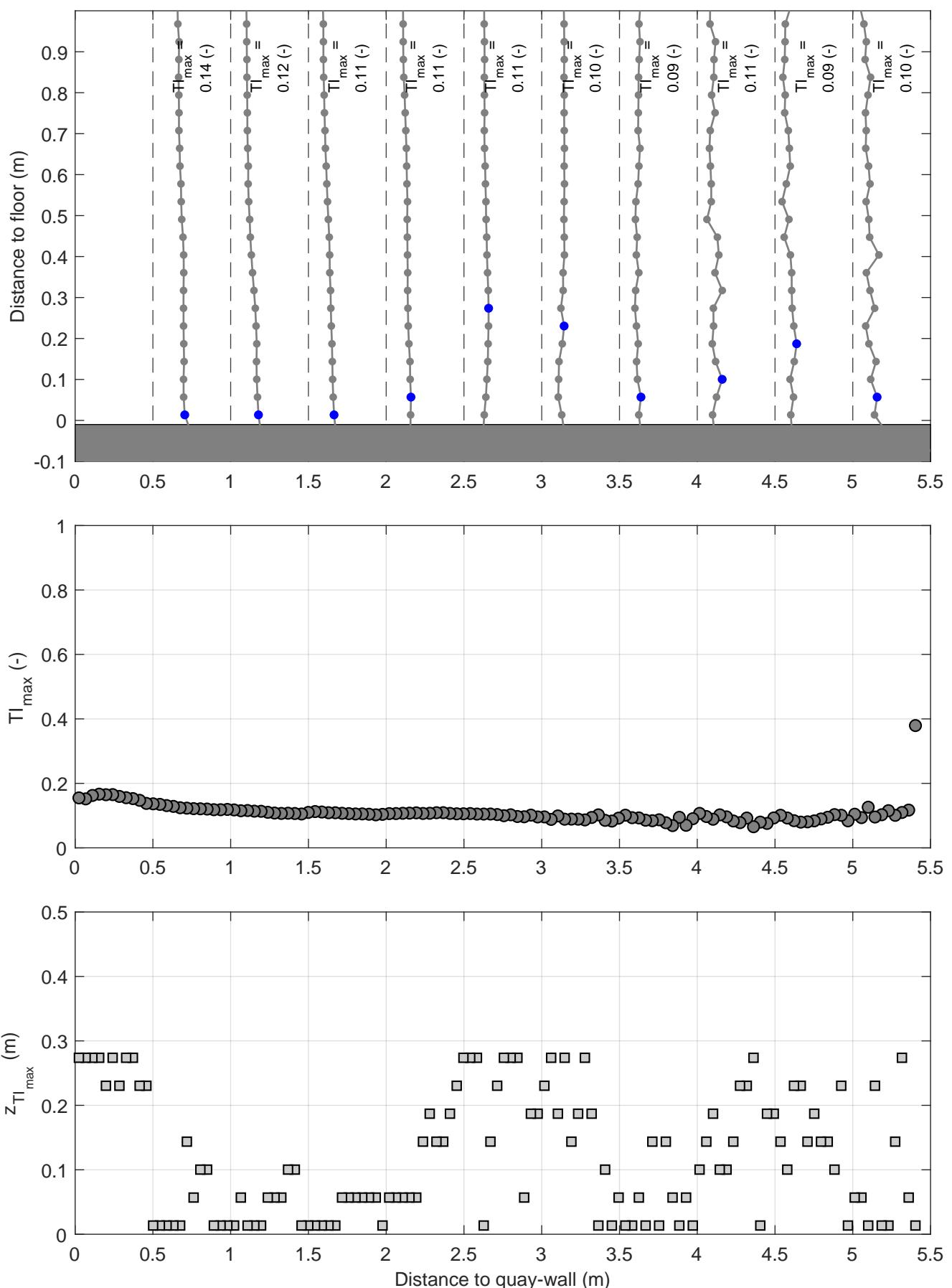
Turbulence intensity profiles | Active thruster: BT2
