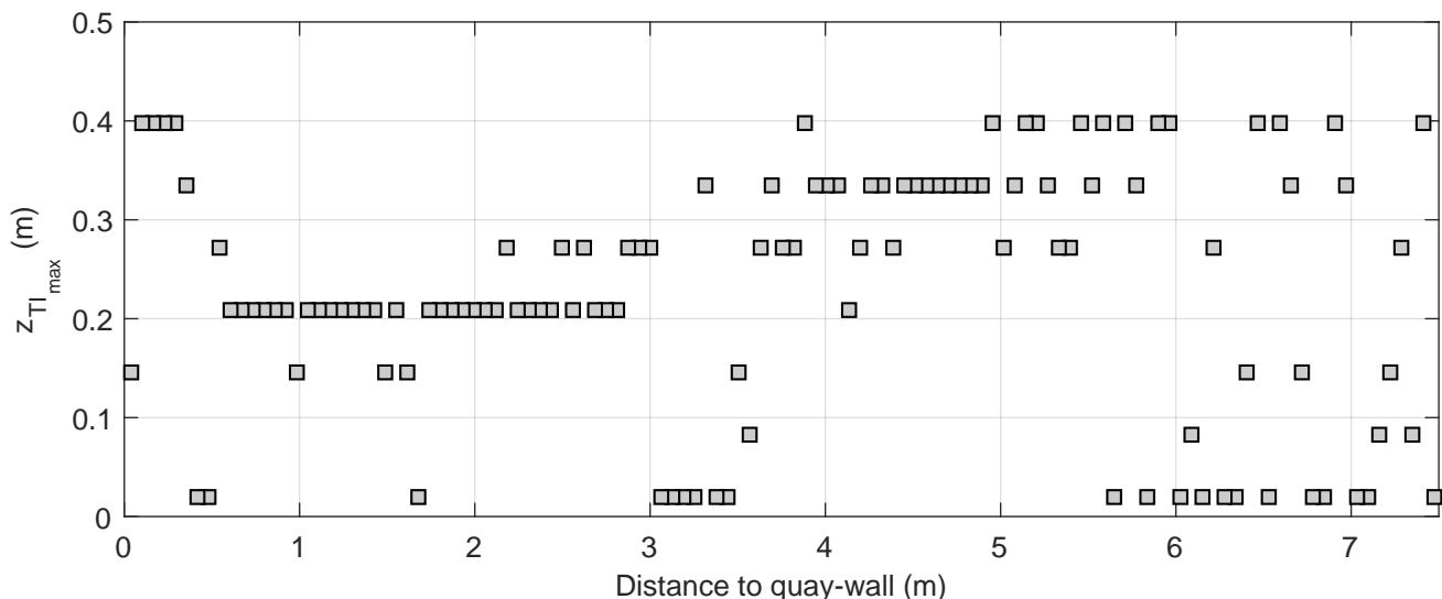
Turbulence intensity profiles | Active thruster: BT2
