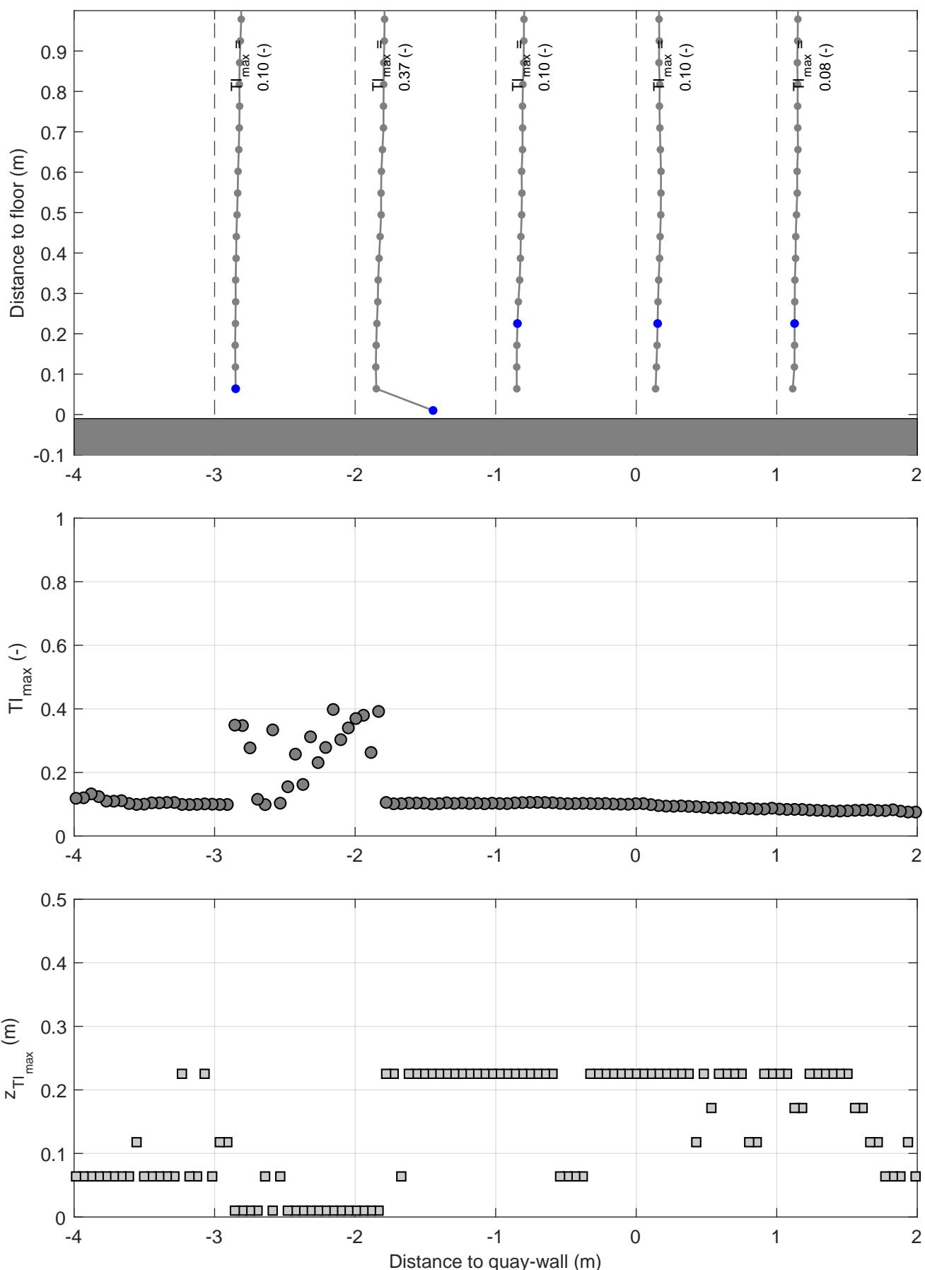
Turbulence intensity profiles | Active thruster: BT2
