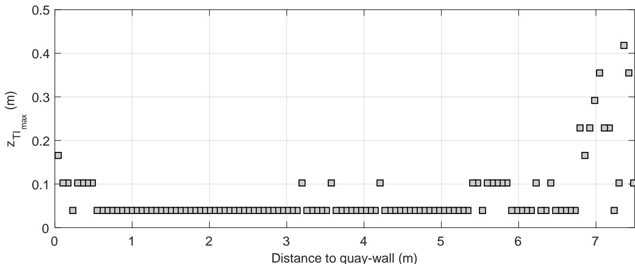
Turbulence intensity profiles | Active thruster: BT1&BT2
