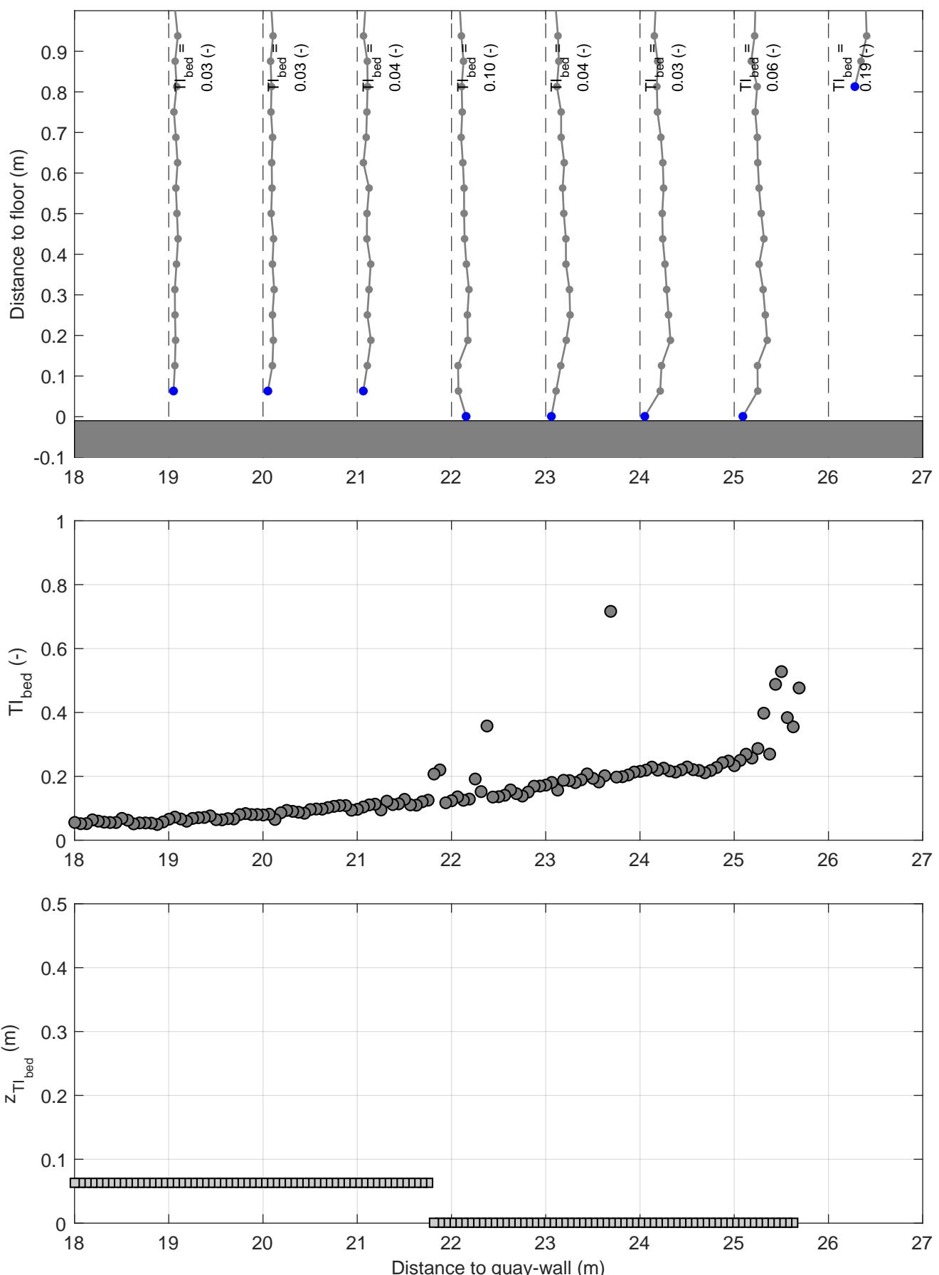
Turbulence intensity profiles | Active thruster: BT1&BT2
