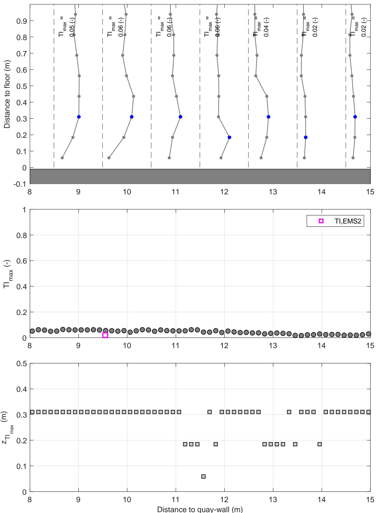
Turbulence intensity profiles | Active thruster: BT2
