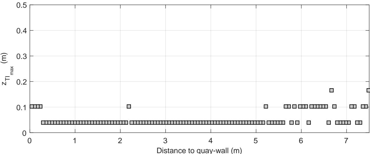
Turbulence intensity profiles | Active thruster: BT1&BT2
