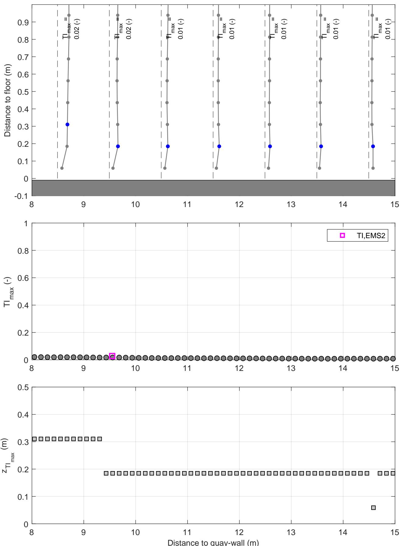
Turbulence intensity profiles | Active thruster: BT2
