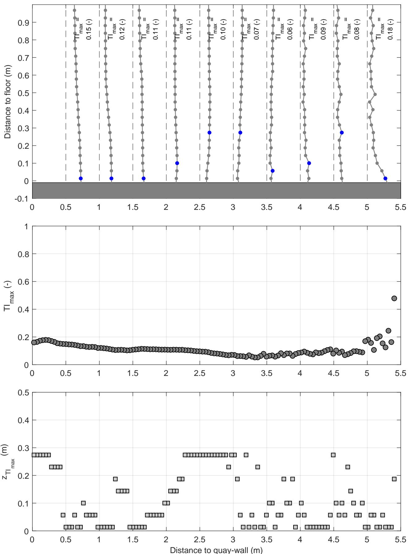
Turbulence intensity profiles | Active thruster: BT2
