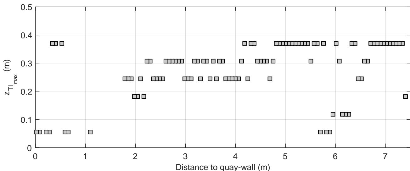
Turbulence intensity profiles | Active thruster: BT2
