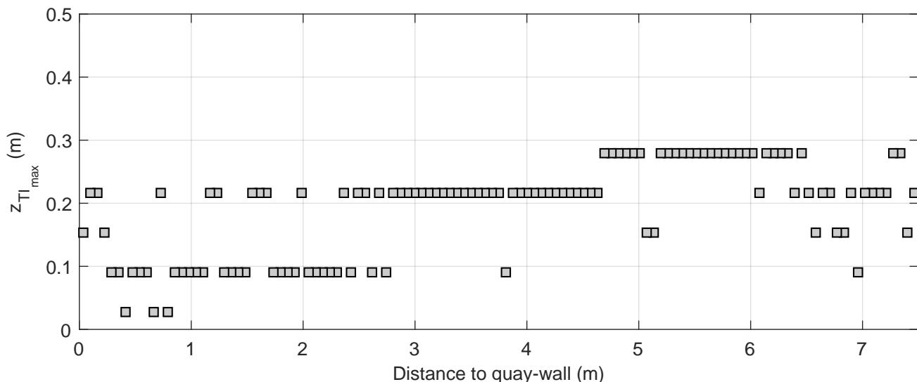
Turbulence intensity profiles | Active thruster: BT1&BT2
