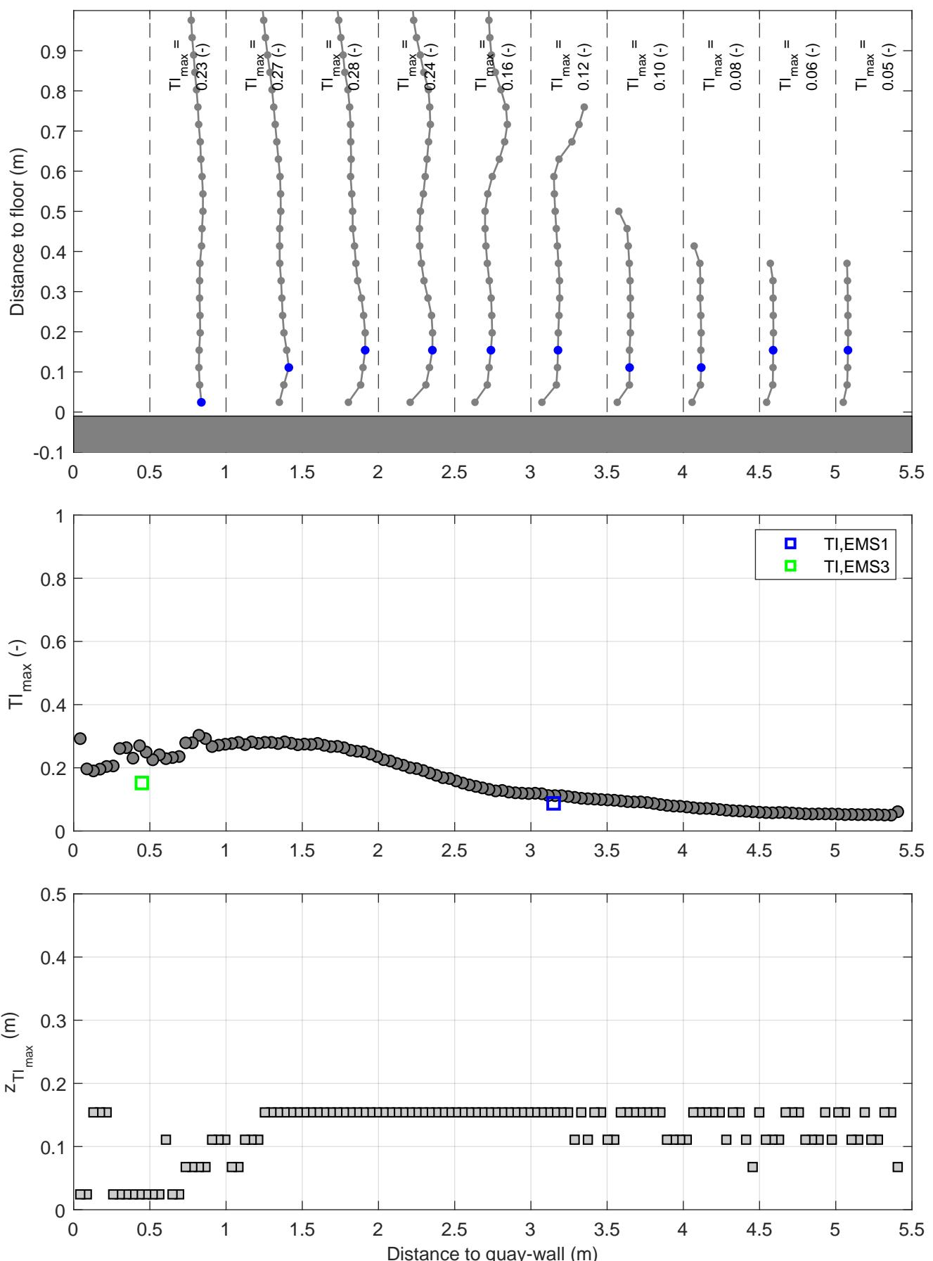
Turbulence intensity profiles | Active thruster: BT2
