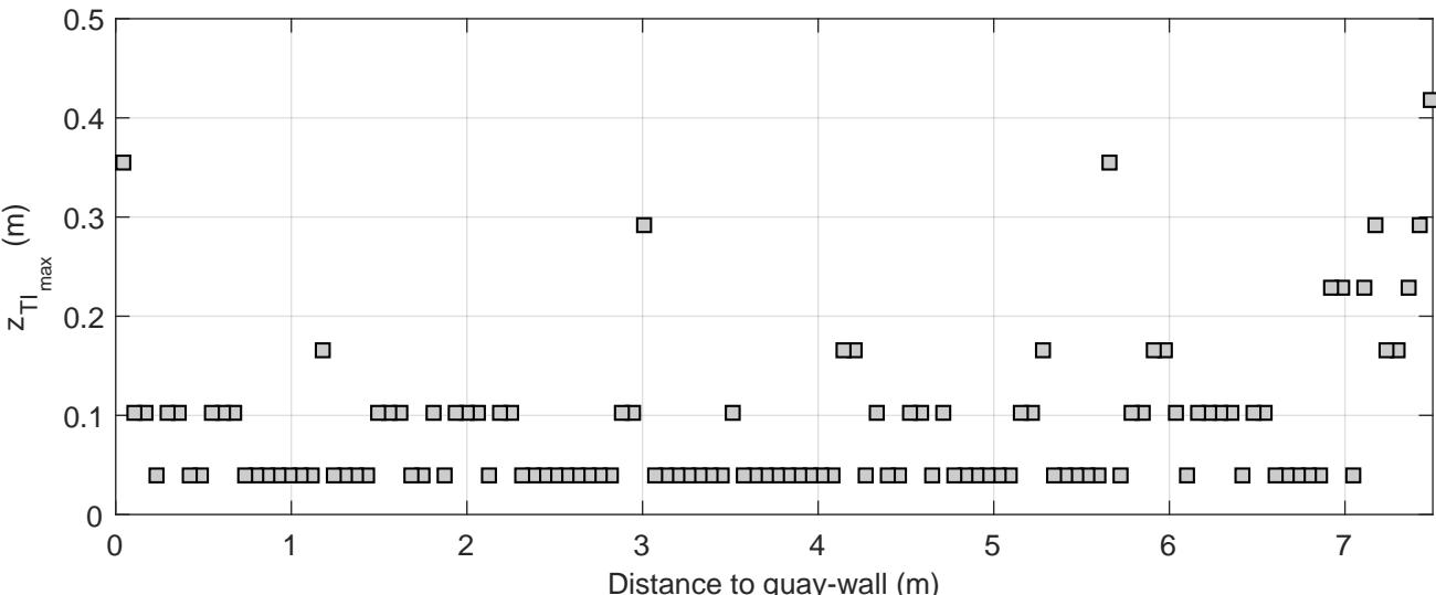
Turbulence intensity profiles | Active thruster: BT1
