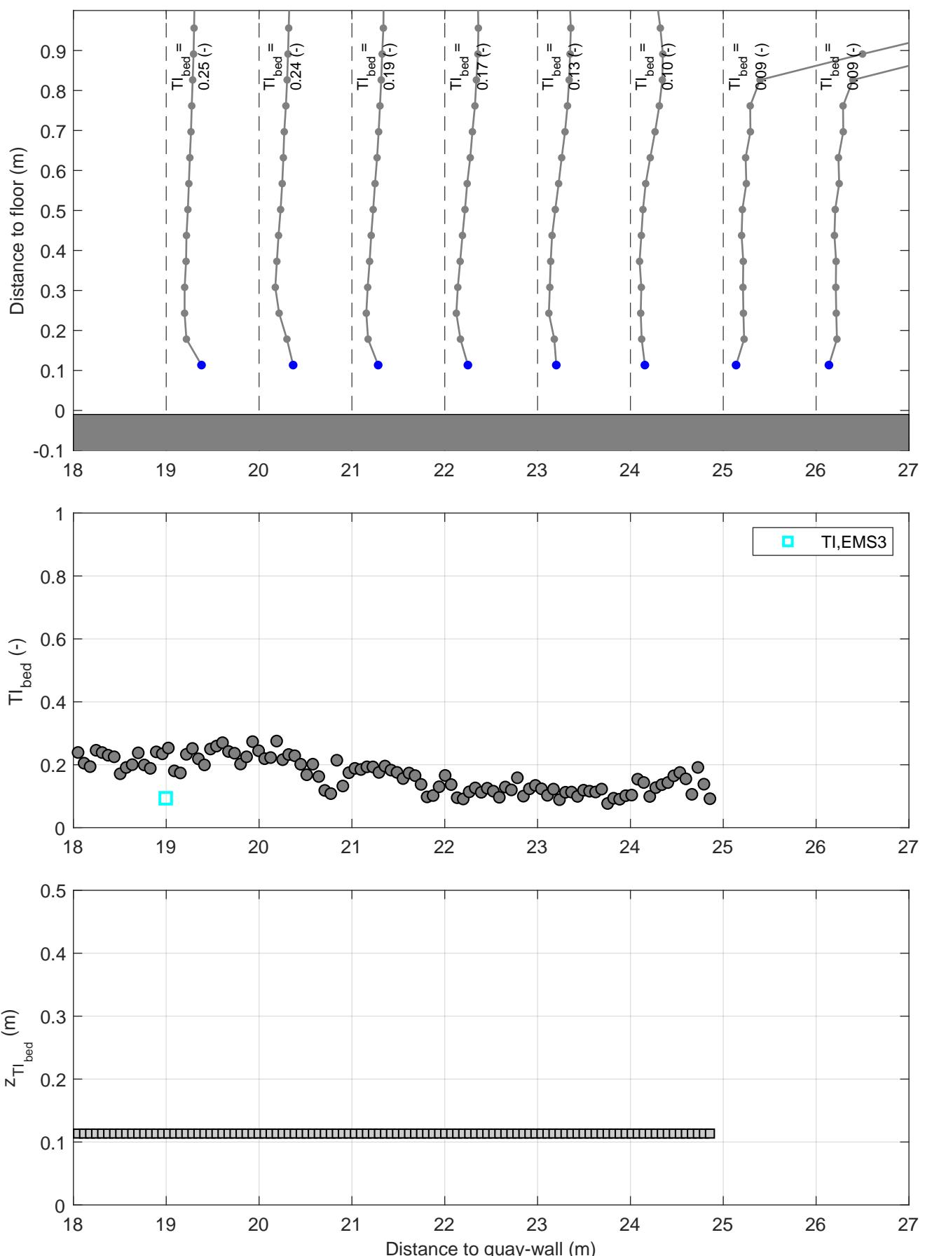
Turbulence intensity profiles | Active thruster: BT2
