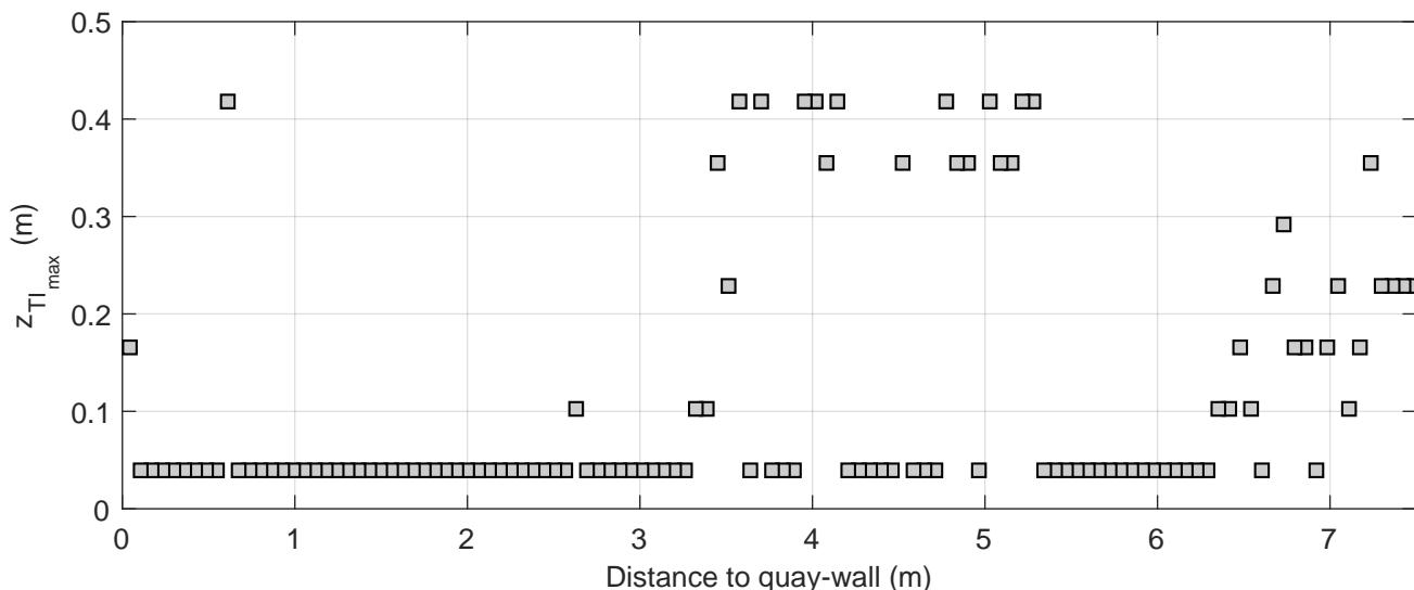
Turbulence intensity profiles | Active thruster: BT1&BT2
