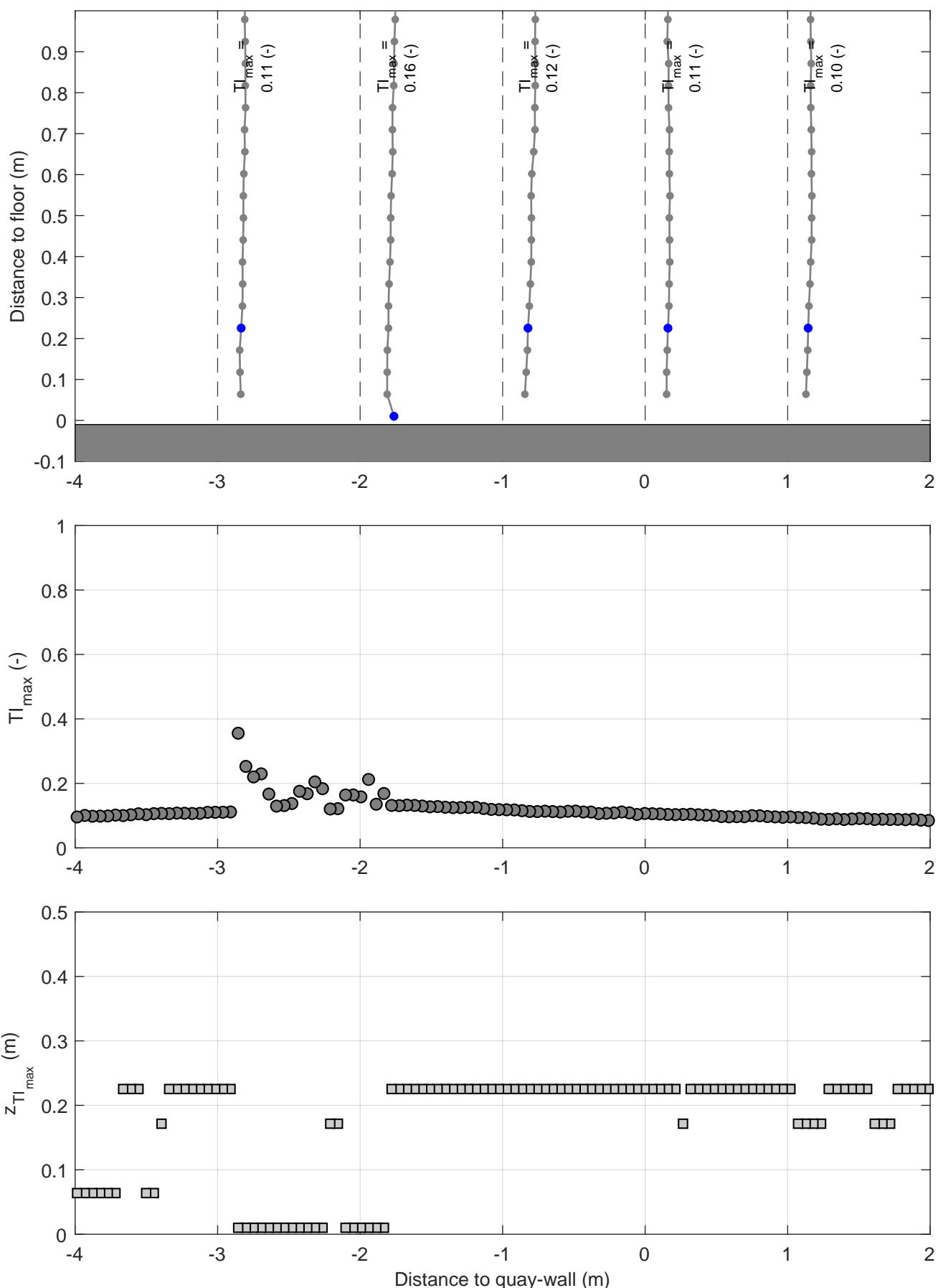
Turbulence intensity profiles | Active thruster: BT2
