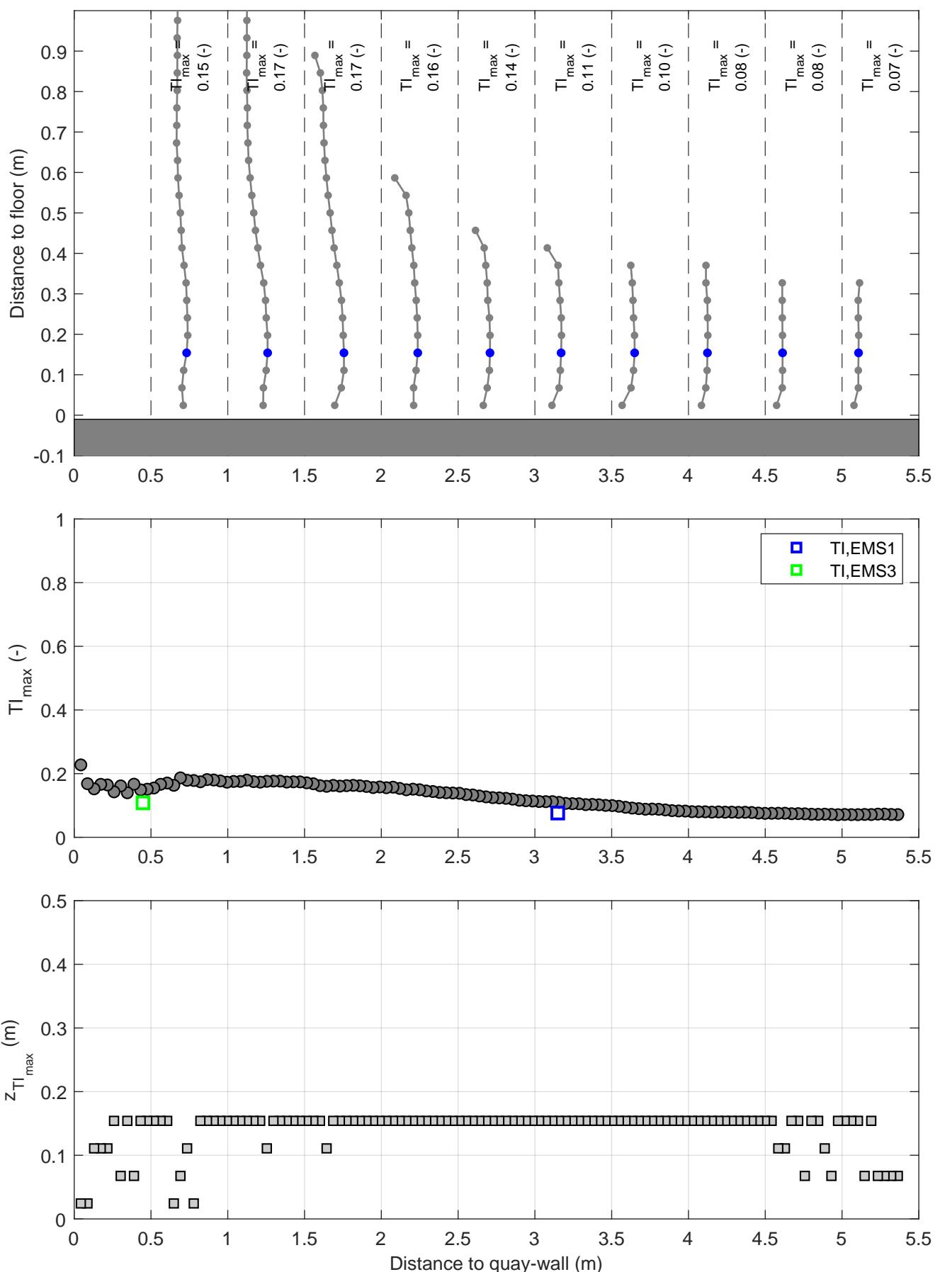
Turbulence intensity profiles | Active thruster: BT2
