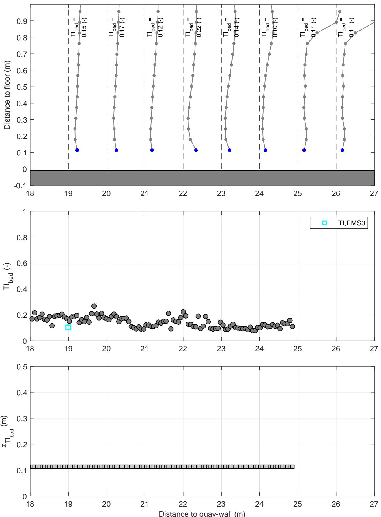
Turbulence intensity profiles | Active thruster: BT2
