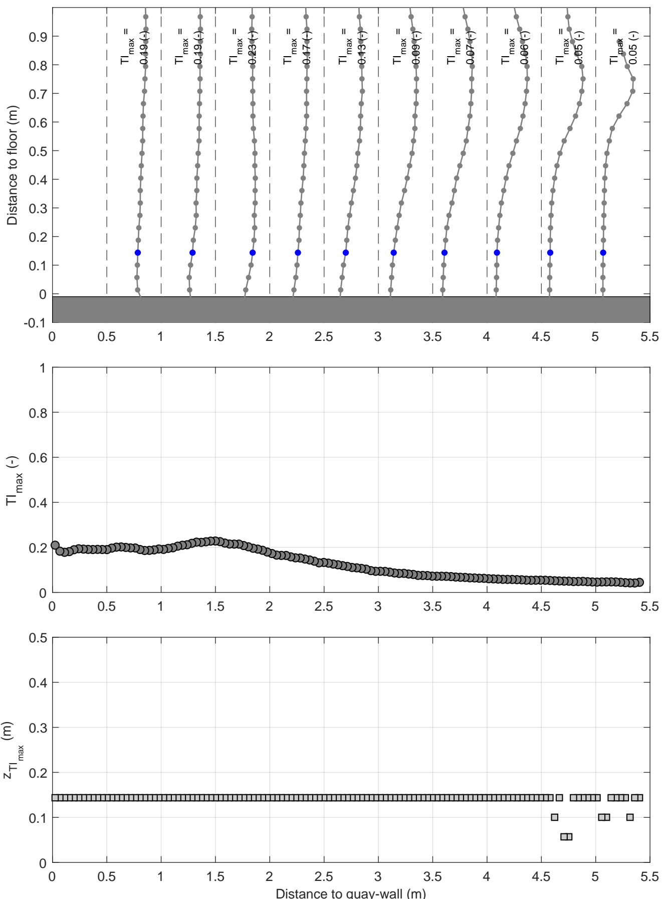
Turbulence intensity profiles | Active thruster: BT2
