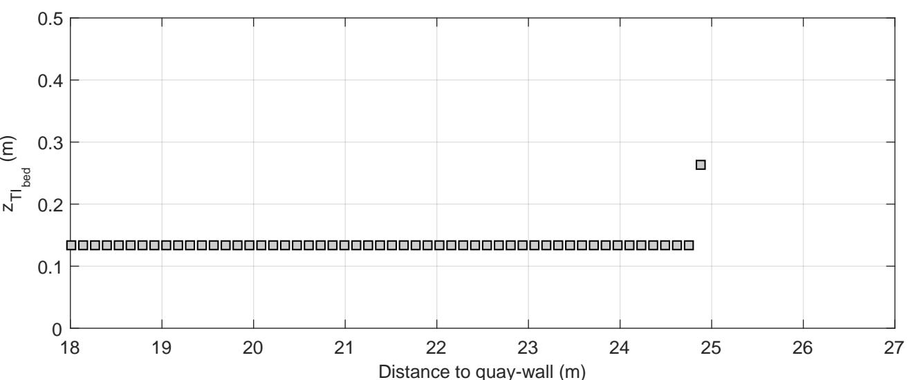
Turbulence intensity profiles | Active thruster: BT2
