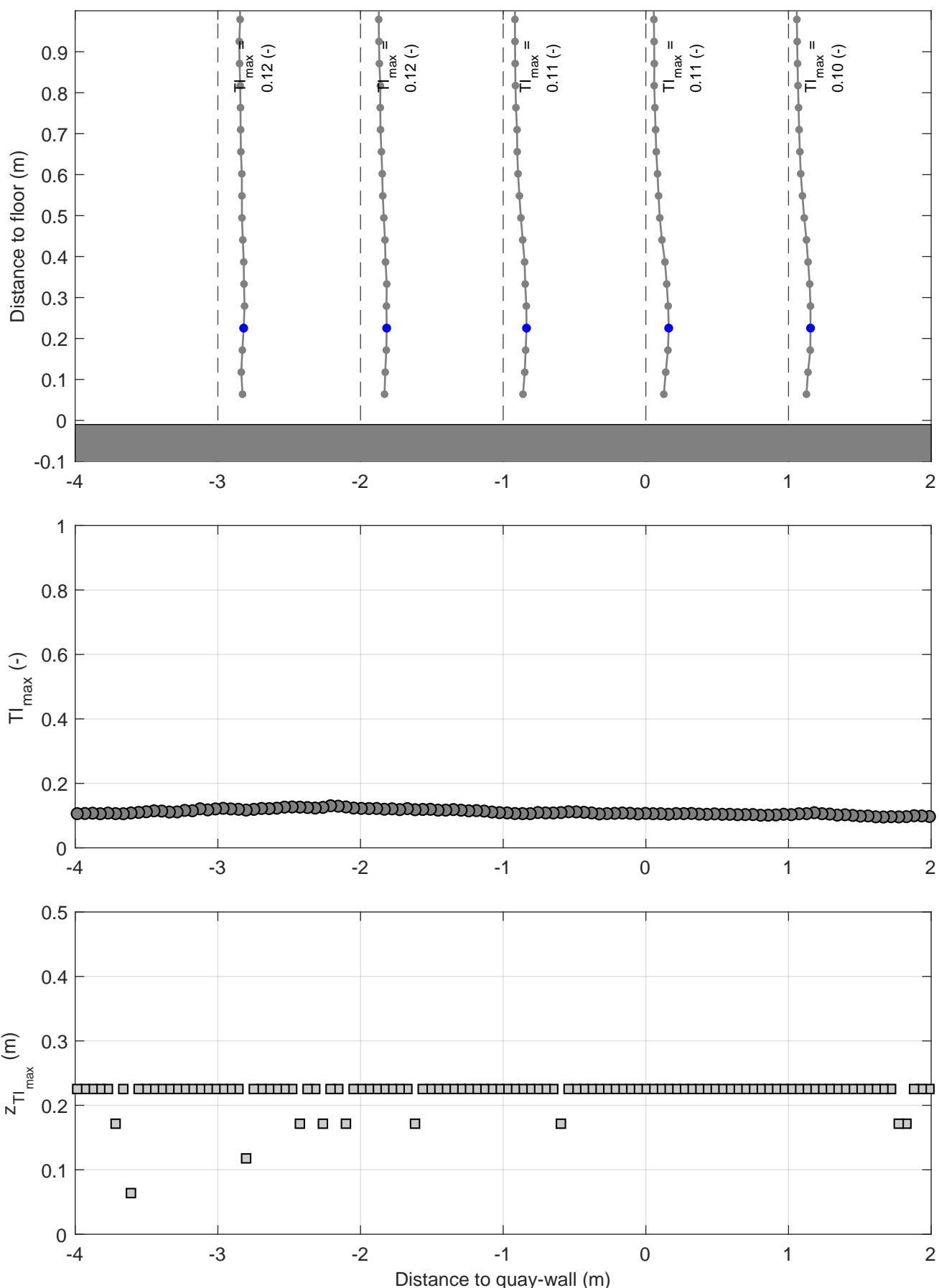
Turbulence intensity profiles | Active thruster: BT2
