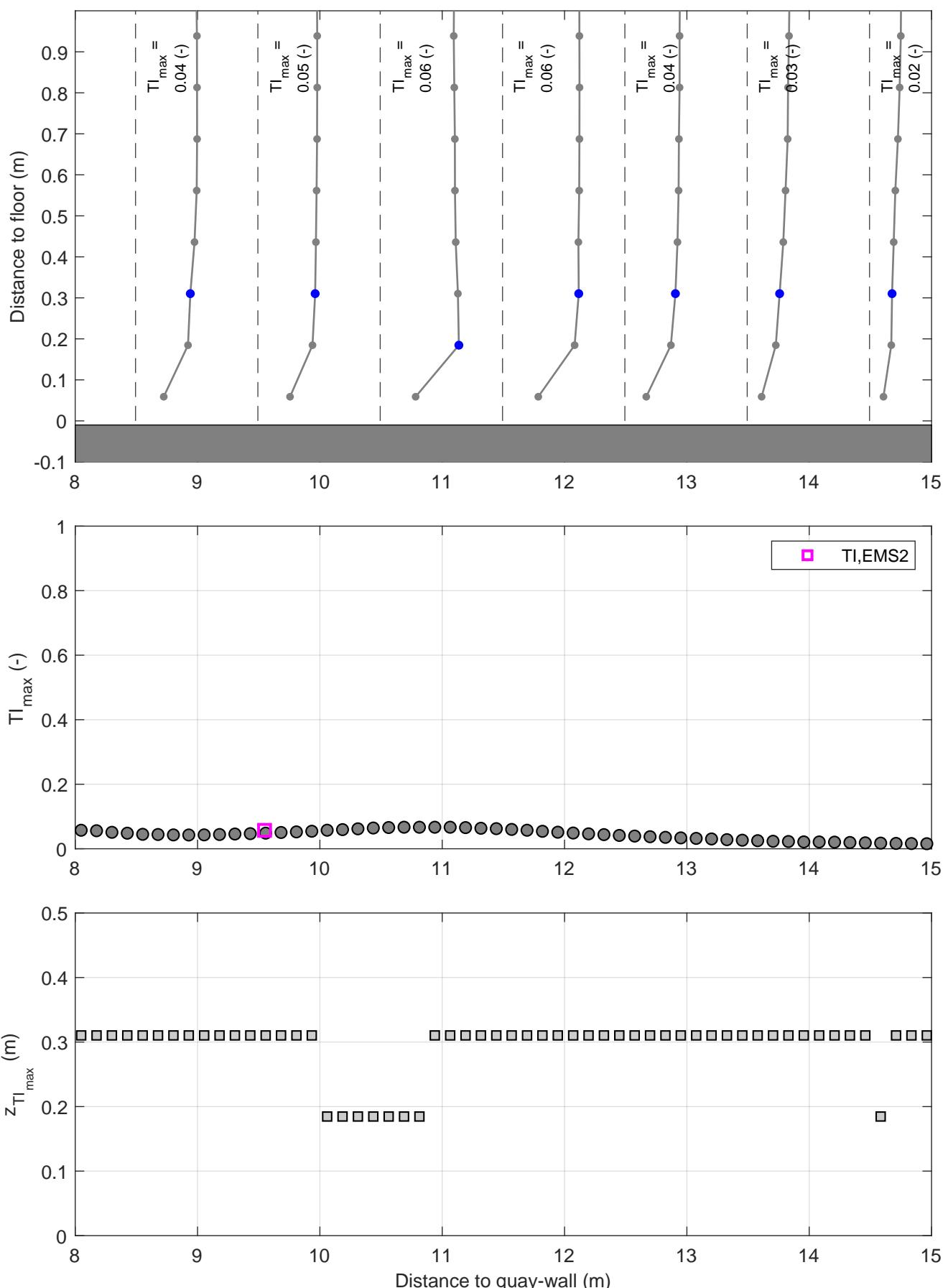
Turbulence intensity profiles | Active thruster: BT2
