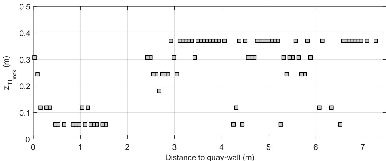
Turbulence intensity profiles | Active thruster: BT2
