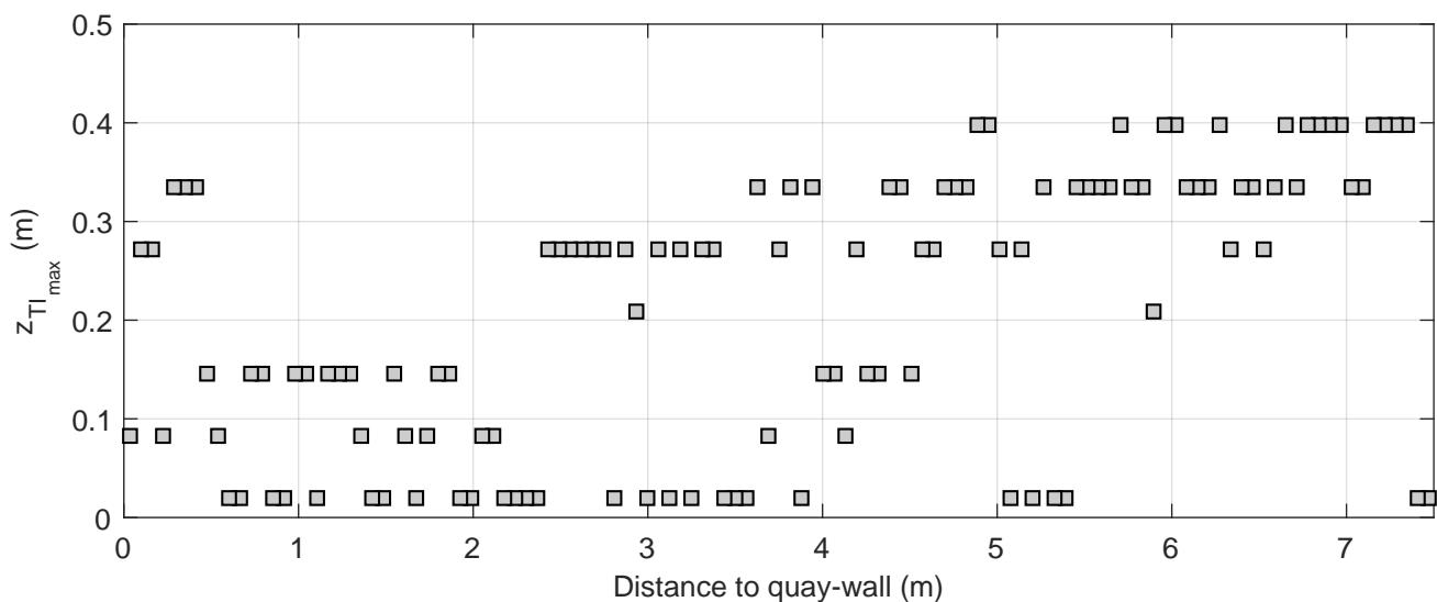
Turbulence intensity profiles | Active thruster: BT2
