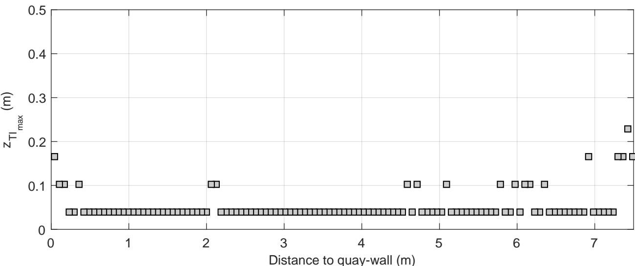
Turbulence intensity profiles | Active thruster: BT1&BT2
