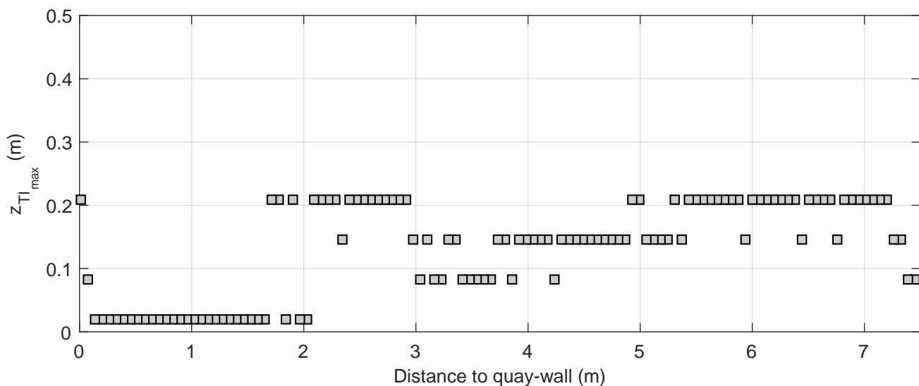
Turbulence intensity profiles | Active thruster: BT2
