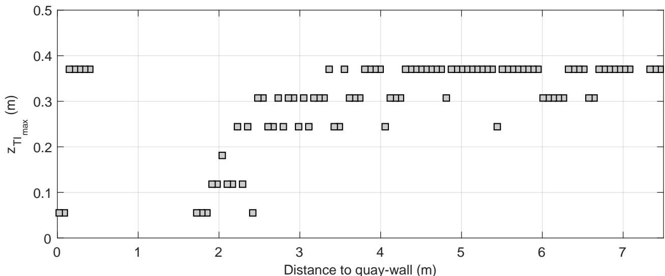
Turbulence intensity profiles | Active thruster: BT2
