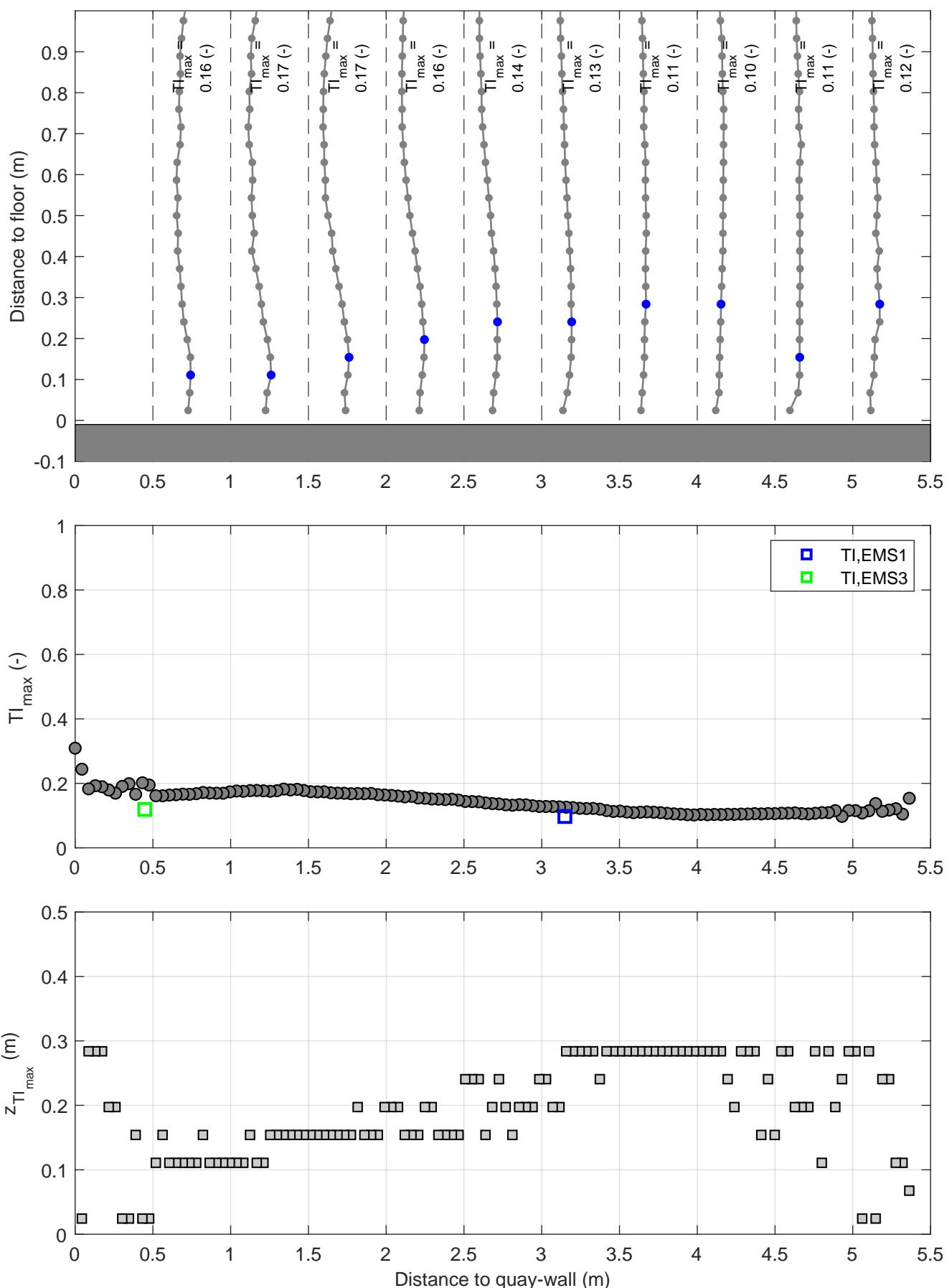
Turbulence intensity profiles | Active thruster: BT2
