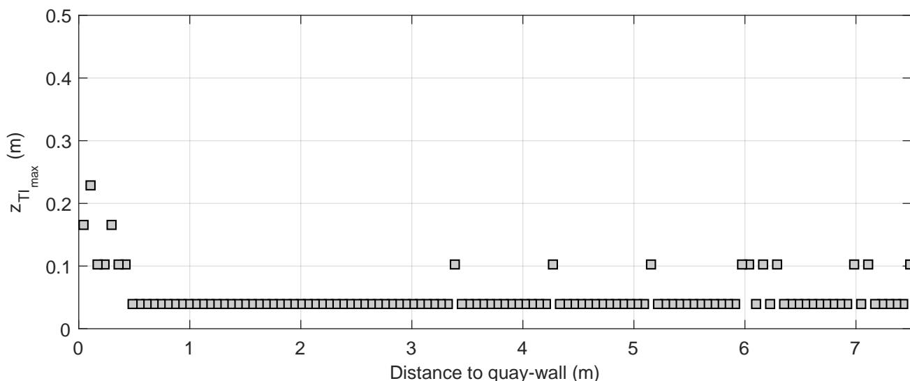
Turbulence intensity profiles | Active thruster: BT1&BT2
