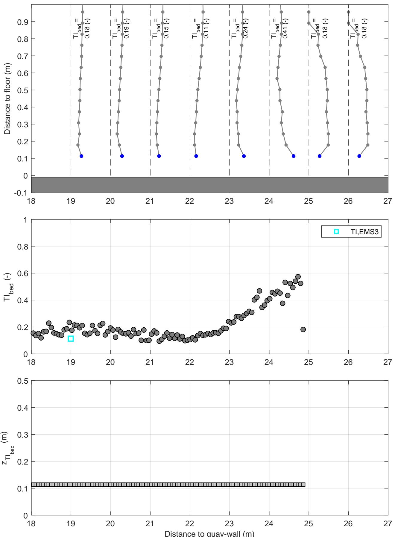
Turbulence intensity profiles | Active thruster: BT2
