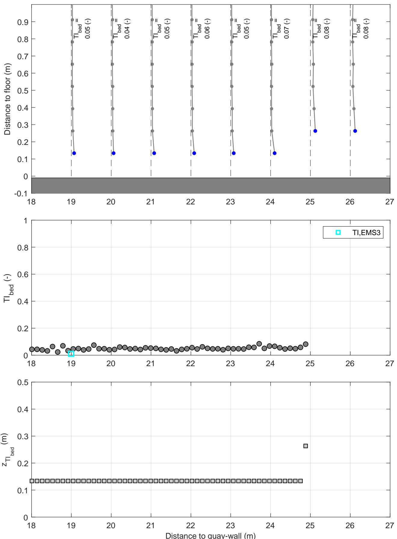
Turbulence intensity profiles | Active thruster: BT2
