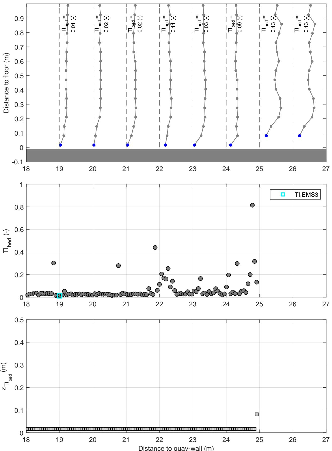
Turbulence intensity profiles | Active thruster: BT2
