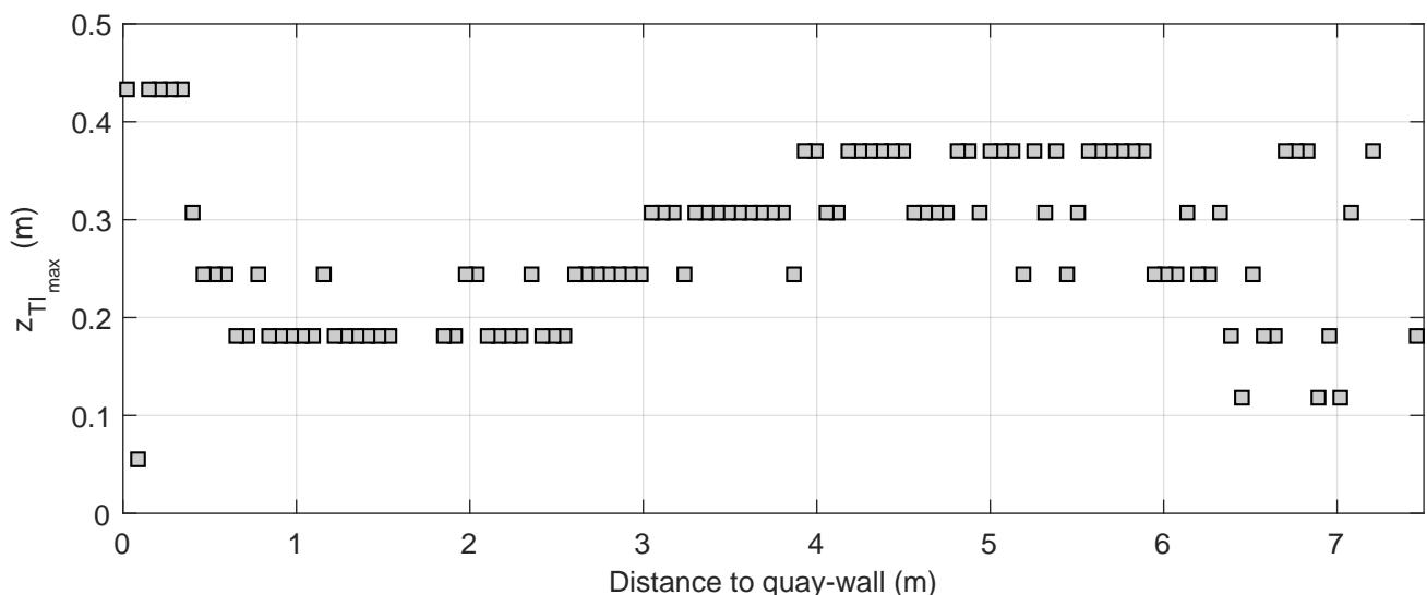
Turbulence intensity profiles | Active thruster: BT2
