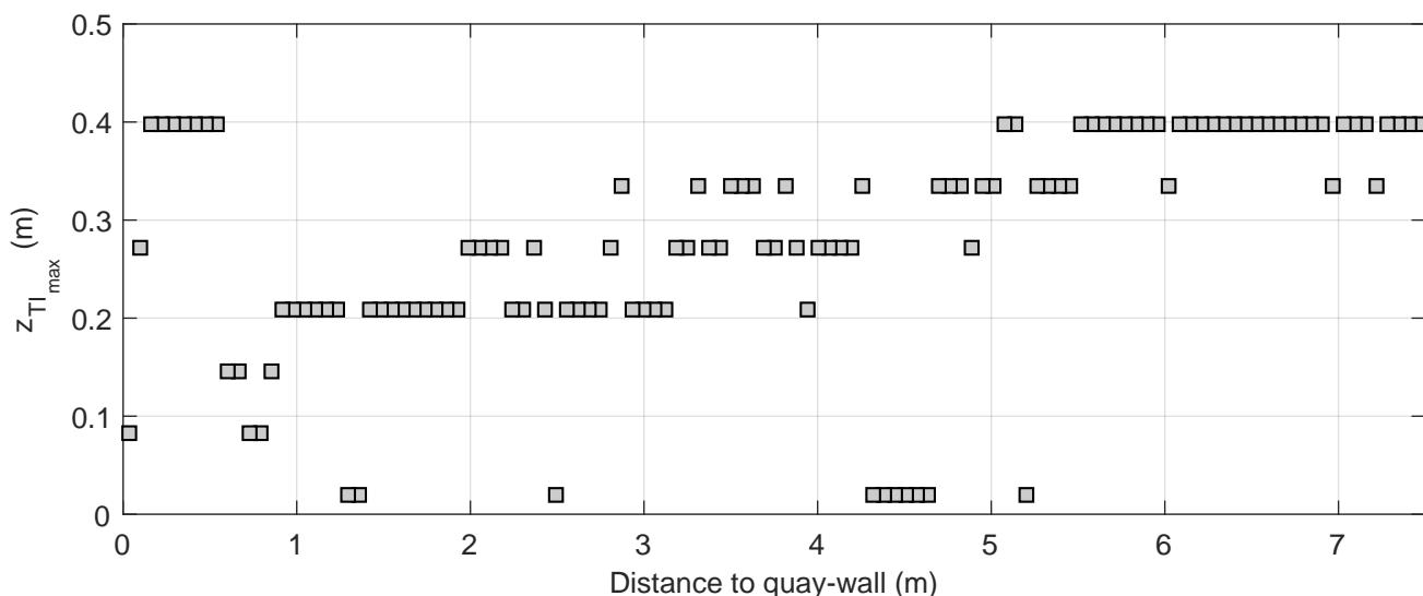
Turbulence intensity profiles | Active thruster: BT2
