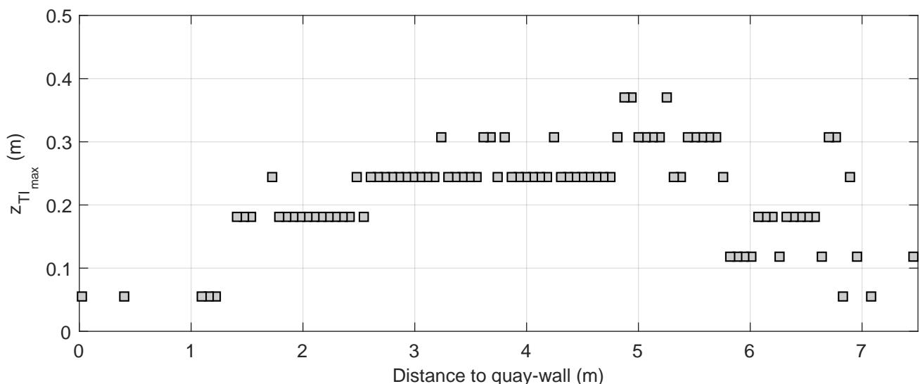
Turbulence intensity profiles | Active thruster: BT2
