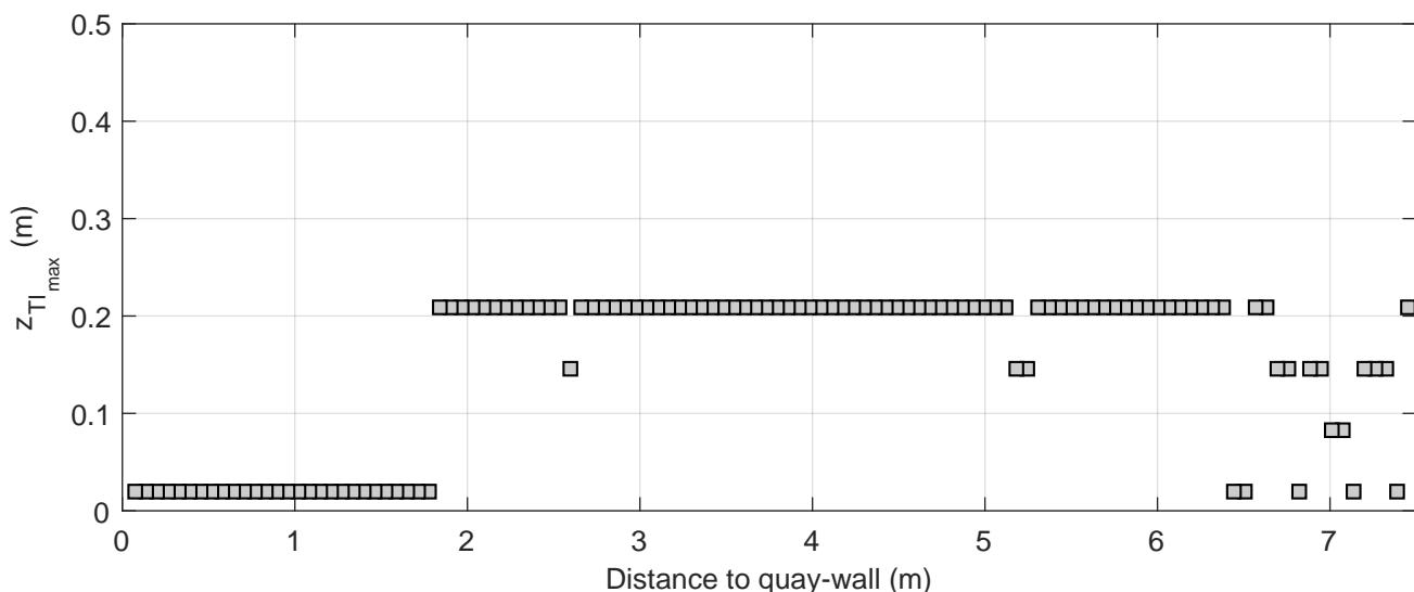
Turbulence intensity profiles | Active thruster: BT2
