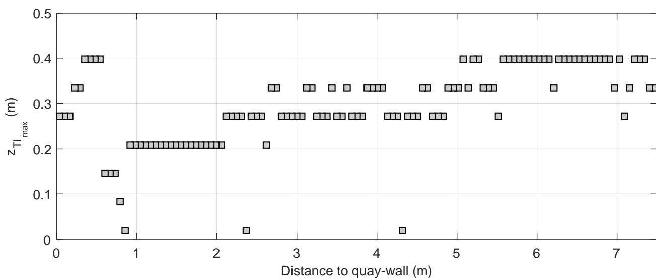
Turbulence intensity profiles | Active thruster: BT2
