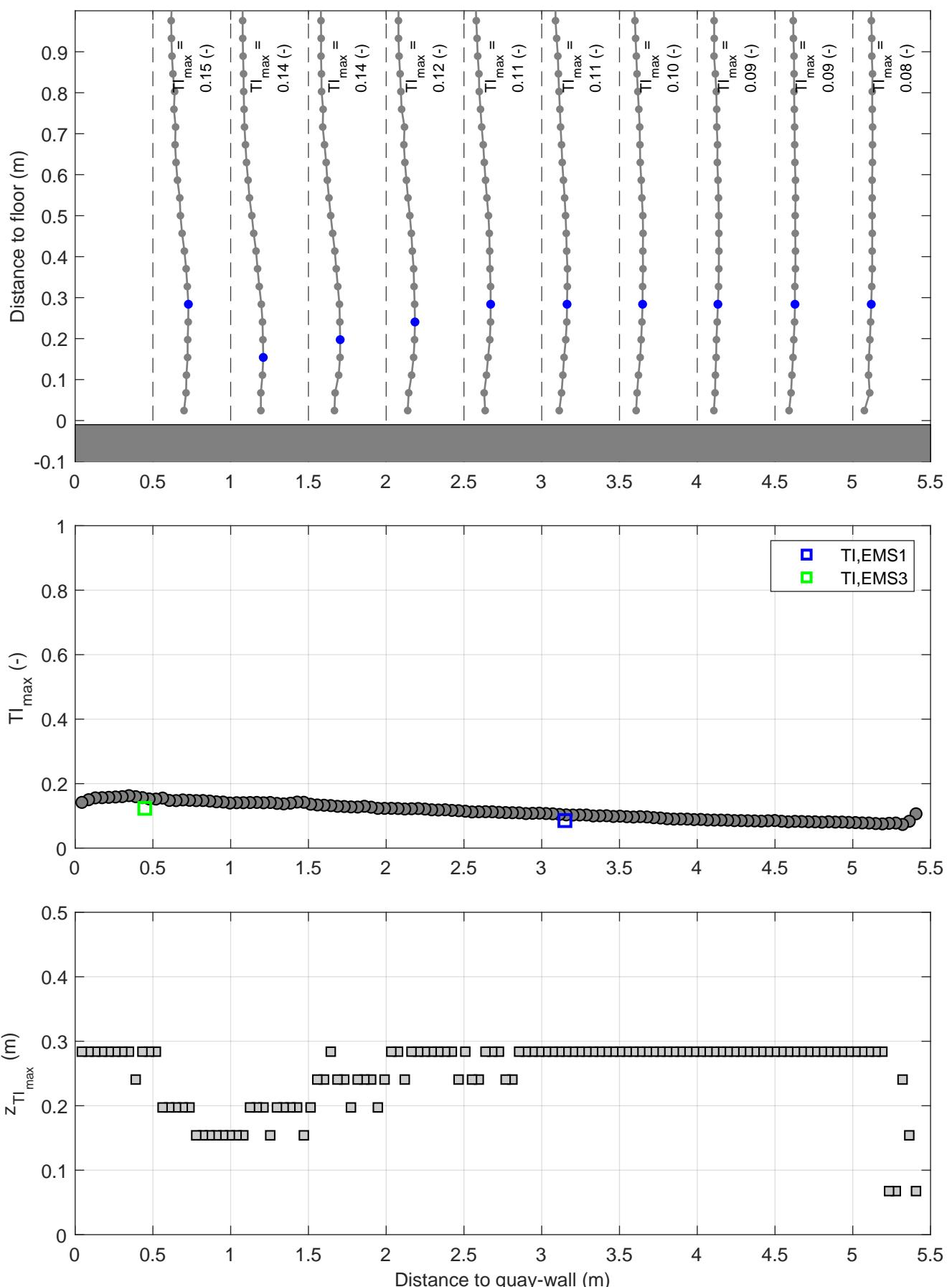
Turbulence intensity profiles | Active thruster: BT2
