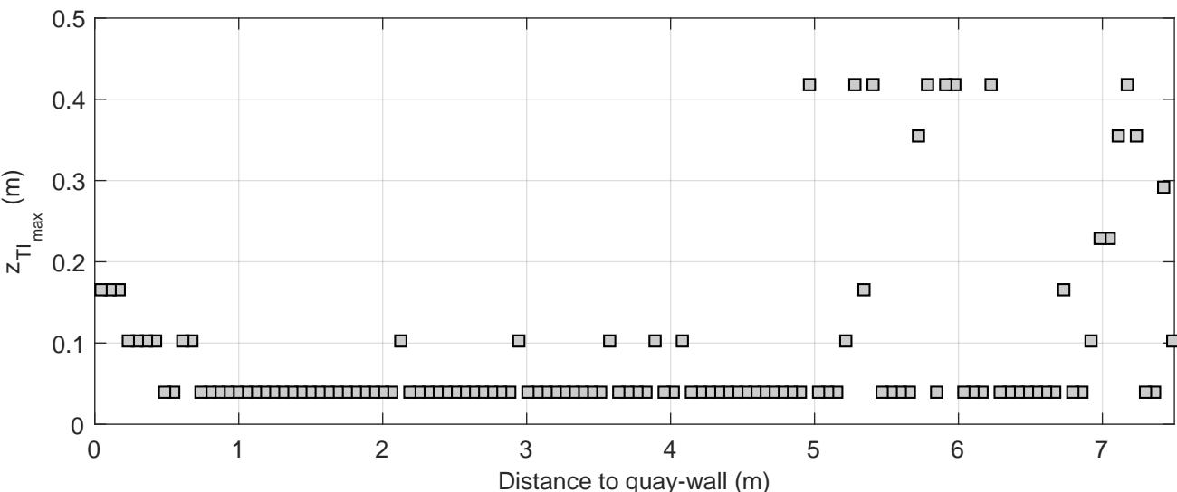
Turbulence intensity profiles | Active thruster: BT1
