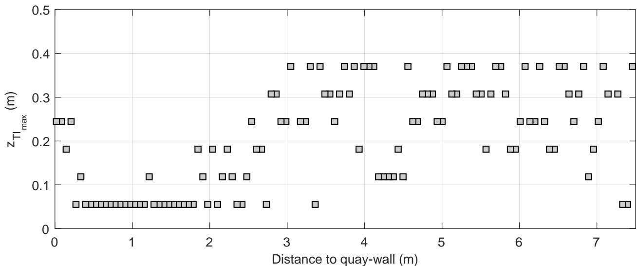
Turbulence intensity profiles | Active thruster: BT2
