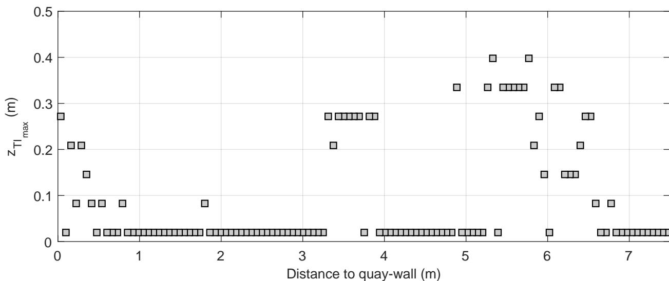
Turbulence intensity profiles | Active thruster: BT2
