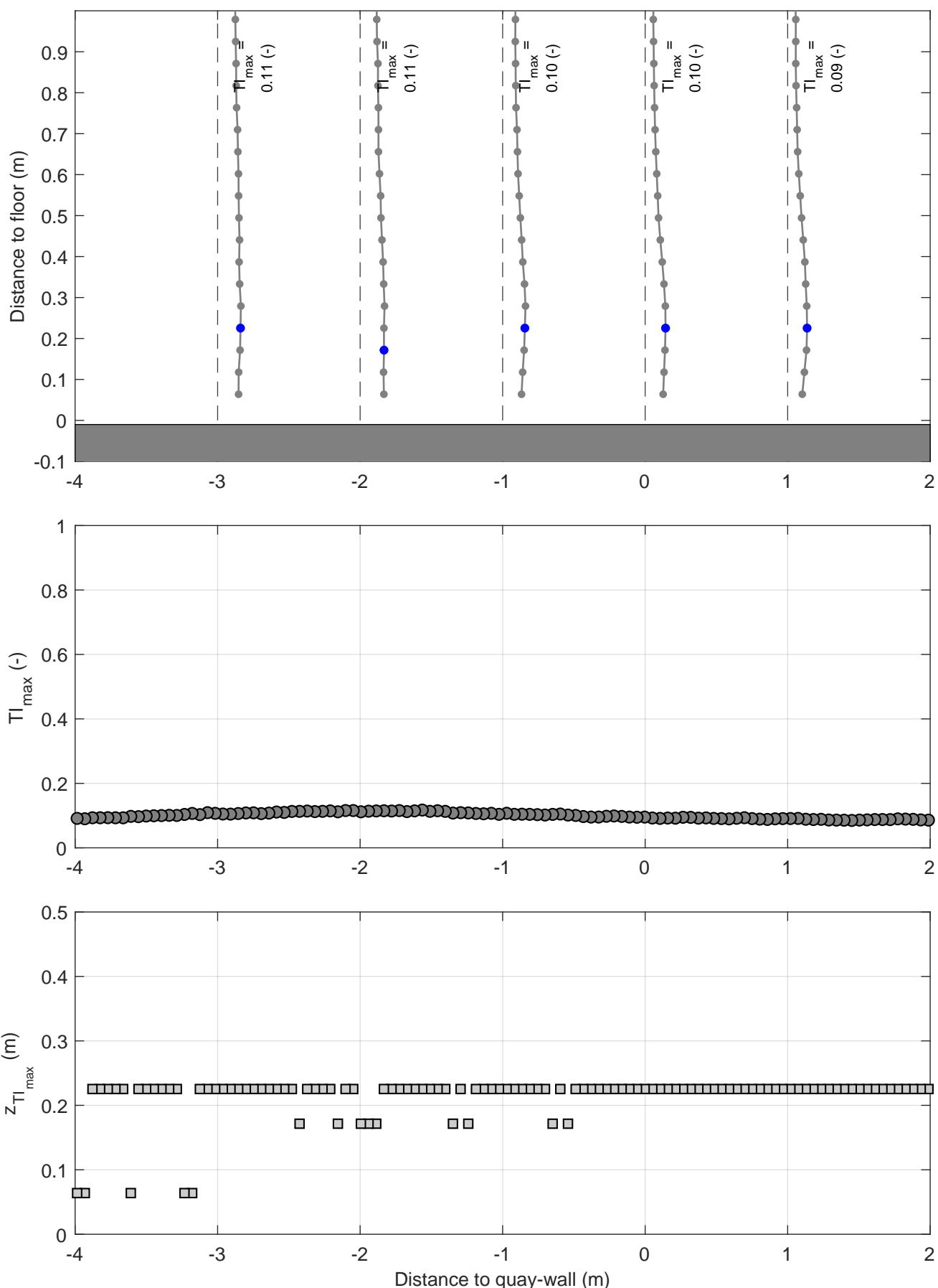
Turbulence intensity profiles | Active thruster: BT2
