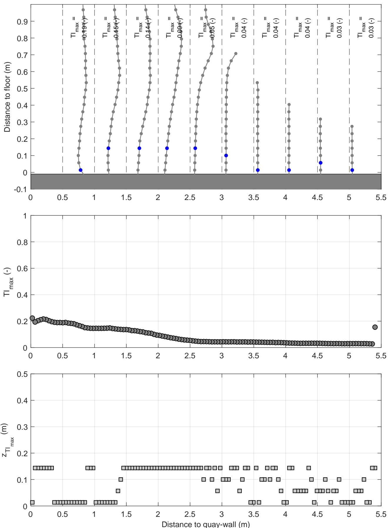
Turbulence intensity profiles | Active thruster: BT2
