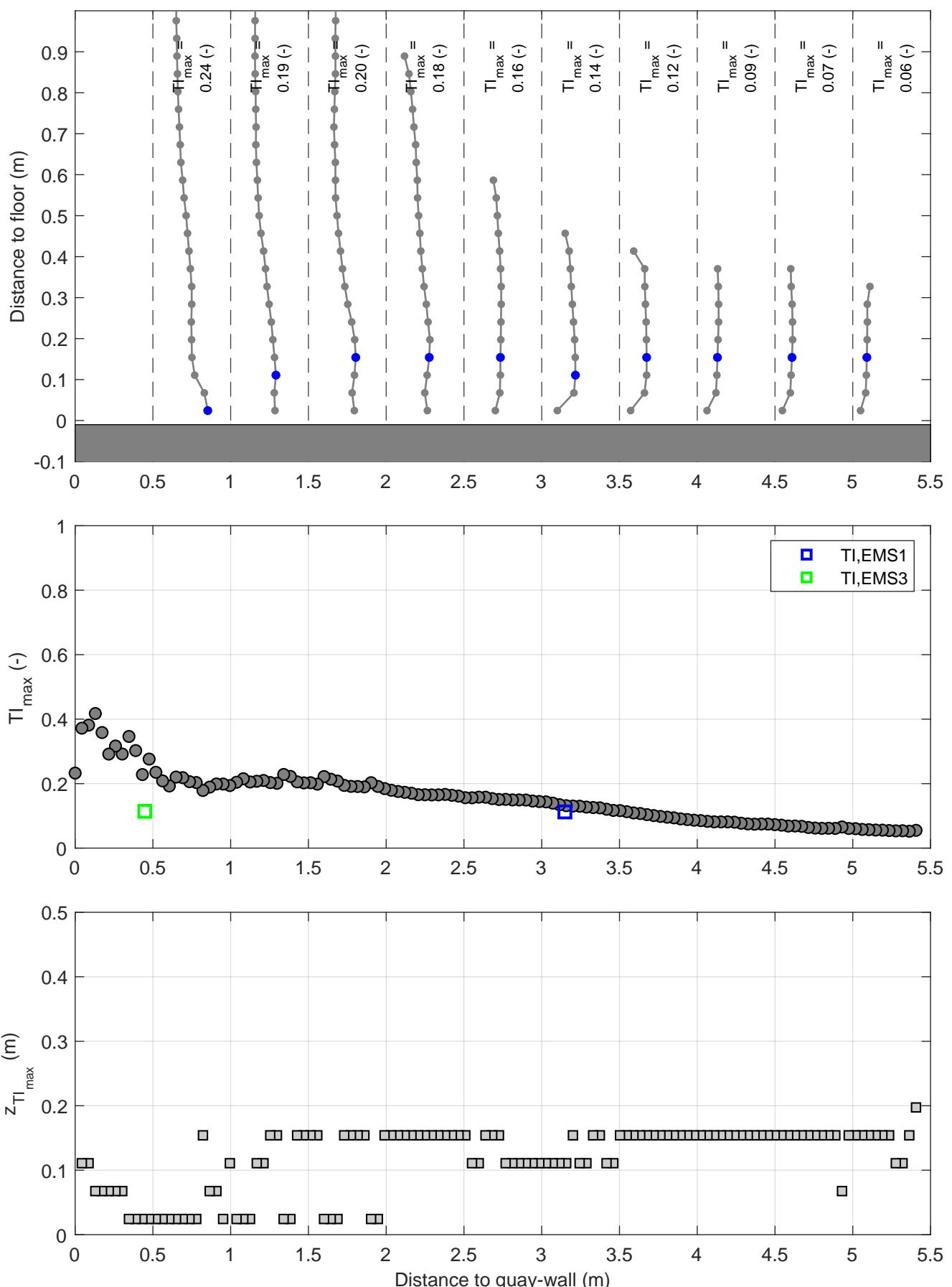
Turbulence intensity profiles | Active thruster: BT2
