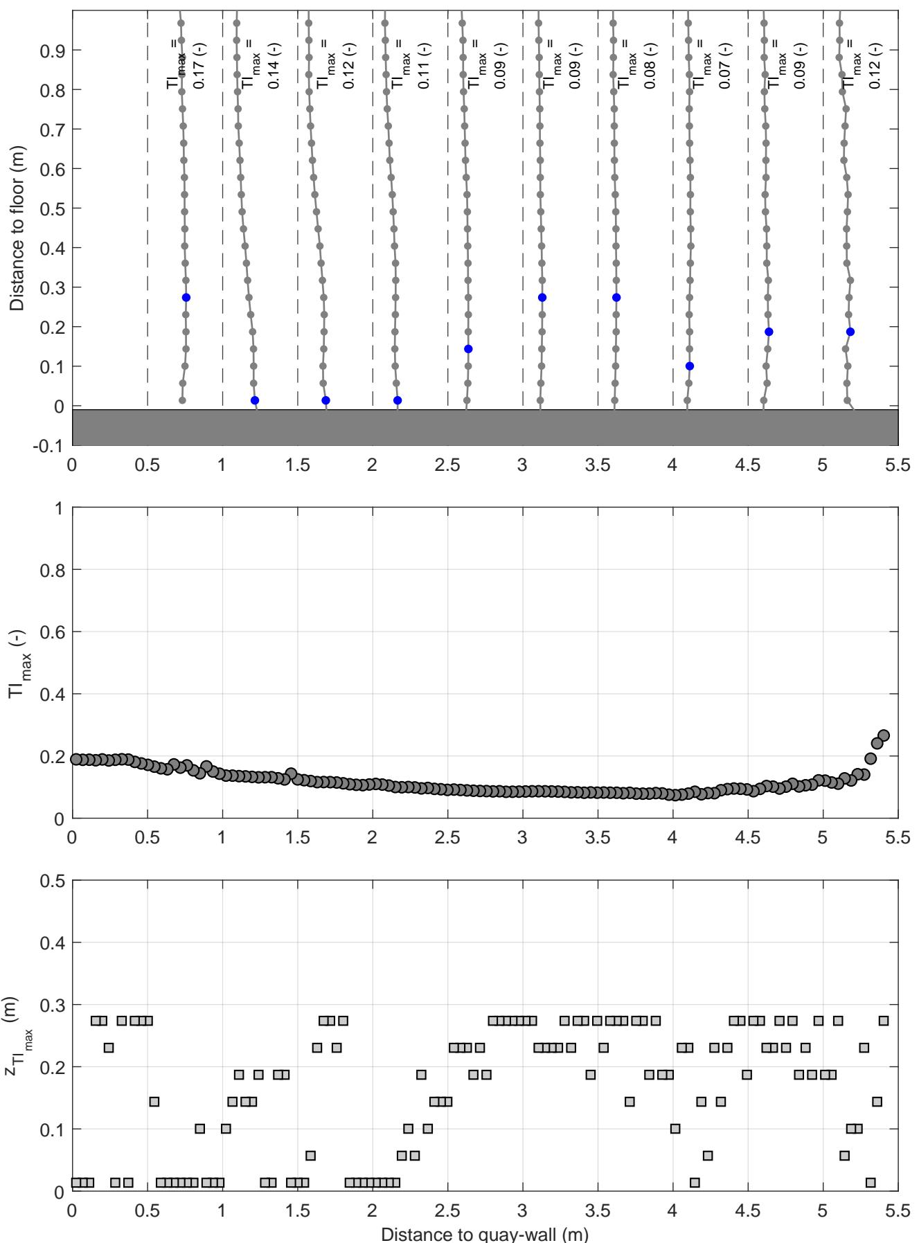
Turbulence intensity profiles | Active thruster: BT2
