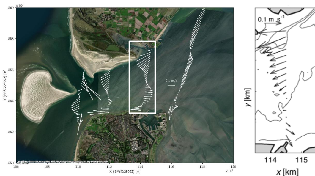
Figure 15 Modelled tidal-mean current through the Marsdiep tidal inlet, computed by averaging current velocities over one tidal cycle (left) compared to the tidal-mean current measured by Buijsman & Ridderinkhof (2007) (right).
