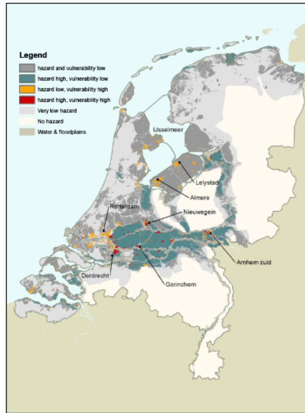
Figure 5 Risky places as overlay of vulnerability and hazard rating.
