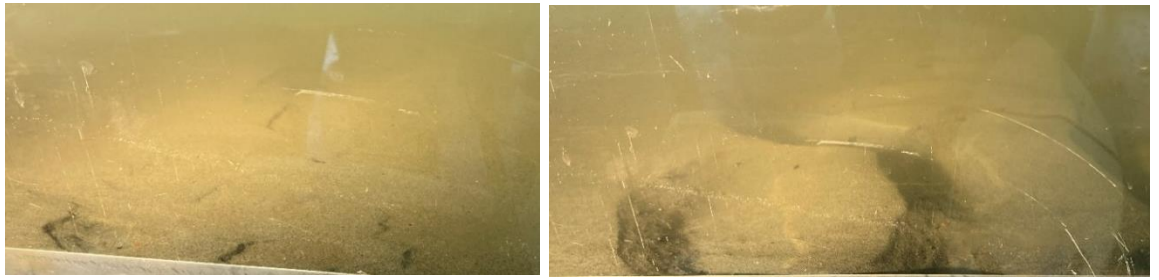
Figure B. 6: Initiation of ripples (left) and growing ripples (right) for test BA-4 ( u_m=0.27 m/s)
