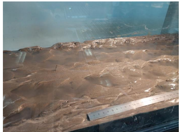
Figure Plan view of bed surface after tests (left) and side view (right); u_m=0.75 ms/, H=0.06 m
