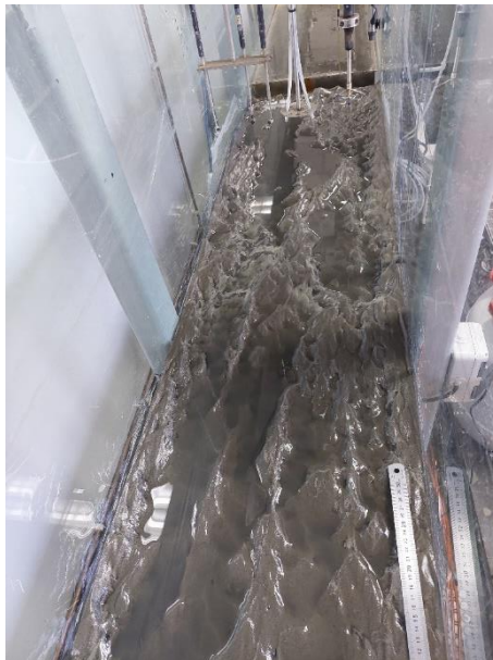
Figure Plan view of bed surface after tests (left) and side view (right); u_m=0.75 ms/, H=0.06 m
