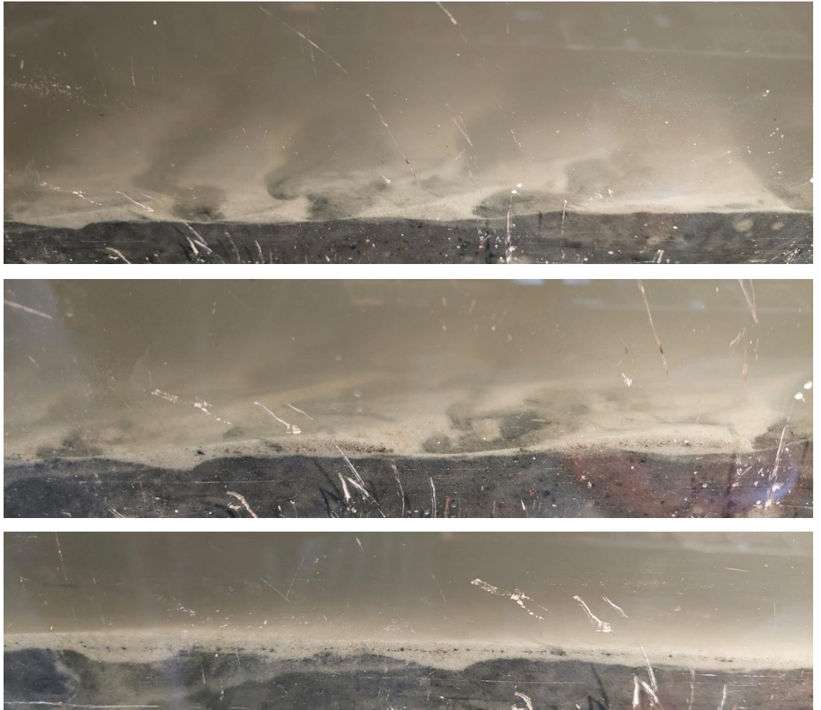
Figure Bed with ripples and sand transport (side view) during combined current+waves
