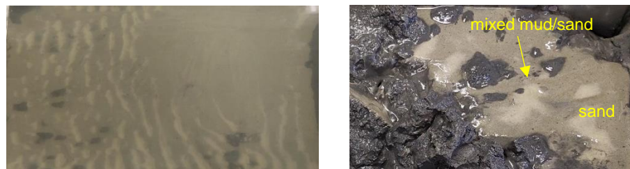
Figure C. 1: Top view bed at end of Test B (light color=sandy crest; grey=silt in ripple troughs; black=deeper mixed mud-sand).
