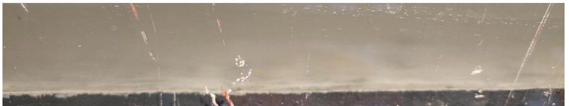
Figure Bed with ripples and sand transport (side view) during combined current+waves
