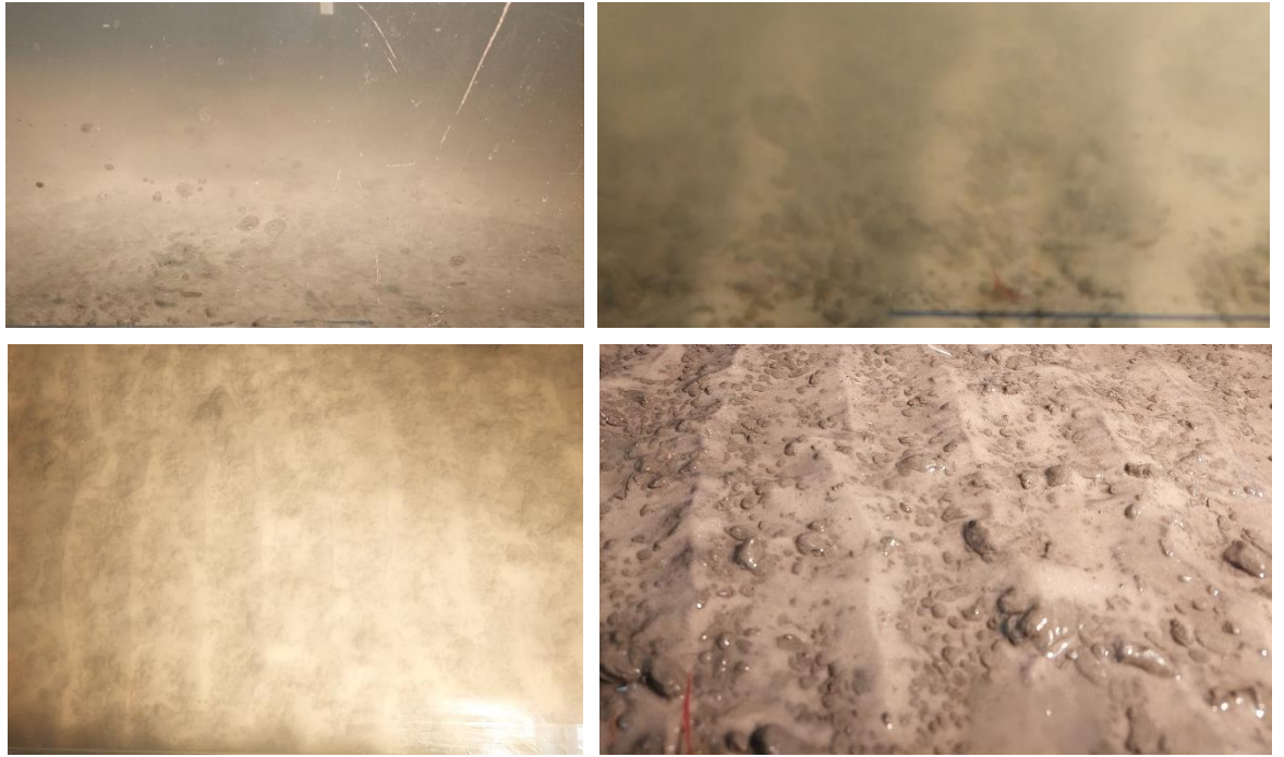
Figure C. 5: Left Upper: Bed before Test D; Right Upper: Bed during Test D (H=12 cm); Left Lower: Top view after Test D; Right Lower: Side view with sand ripples and mud balls (light color=sandy spots; darker grey=finer and mud balls)
