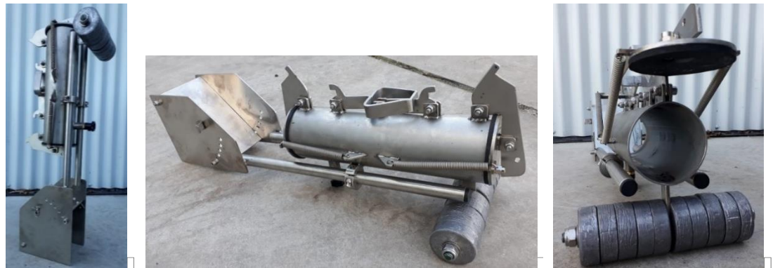
Figure 2.6.6 Pictures of the PIRANHA-instrument, which is used to take samples and to perform settling experiments.
