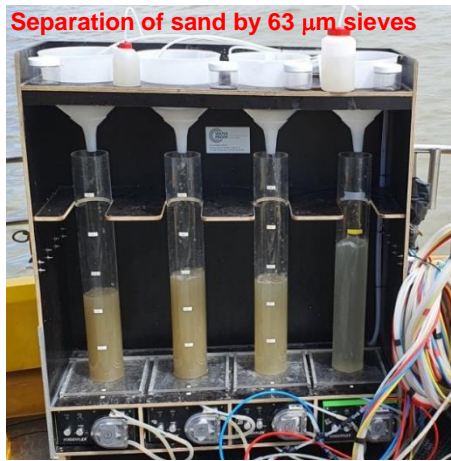
Figure 3.4.6 Measurement frame with intake nozzles and filtration system to determine sand- and mud concentrations.
