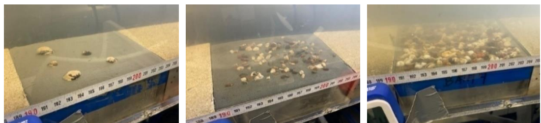
Figure 3.2.8 Flume experiments with short beds and low coverage of shells ( <10\% ; left), a medium coverage of stones (10-20%; middle) and a high coverage of stones (20-40%; right).
