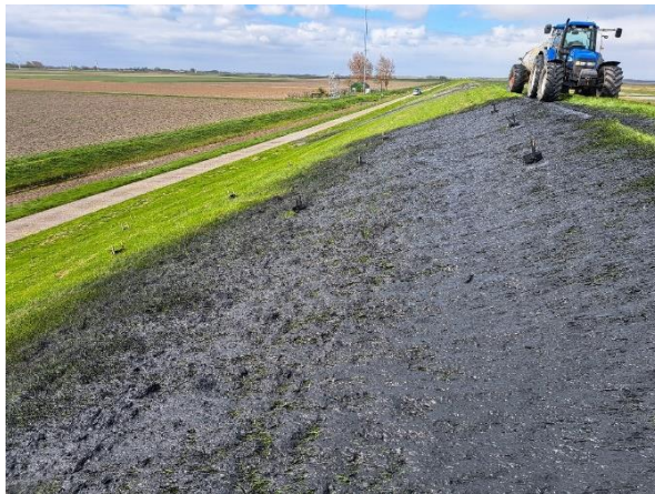
Figure 5.2: Picture from the location of the application experiment during the investigation of the combination(s) between tractor speed and nozzle inclination.
