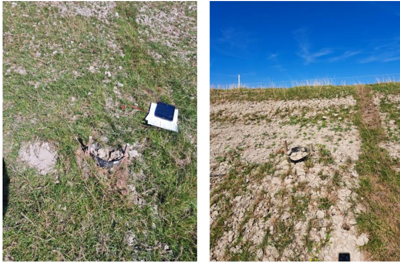
Figure 6.24: Slope three months later the beginning of the pilot. The surface exhibits heterogeneity, with patches characterized by varying degrees of vegetation cover, while others were solely covered by sediment.
