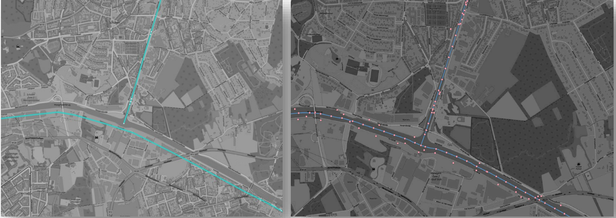
Figure 3 A connection between two waterways. In the FIS network (left), these are not connected correctly and the bottom edge is not properly aligned with the waterway. The connection in EuRIS does not have this issue.
