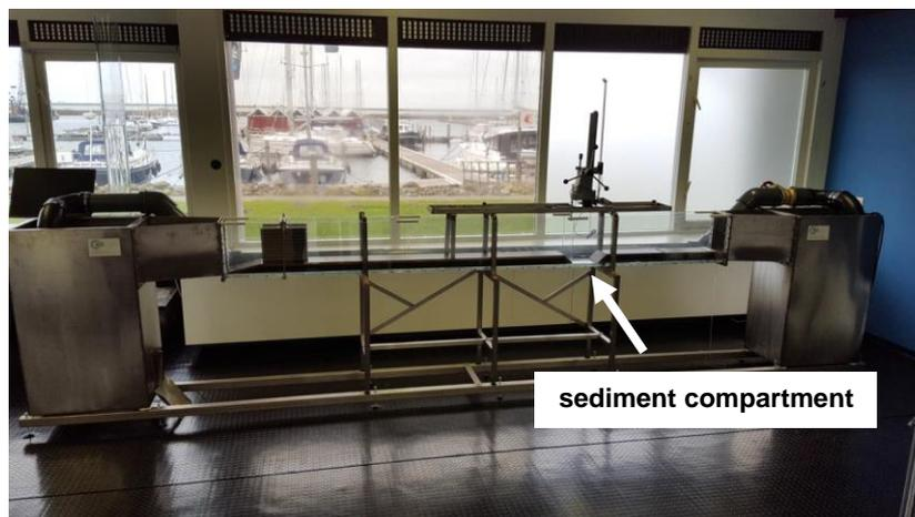
Figure 2-7 Small flume in the laboratory of WaterProof. The flow direction in the flume is from left to right in the picture. The sediment sample is placed in the central section of the flume.
