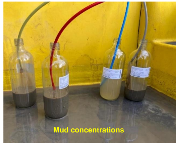
Figure 3.4.6 Measurement frame with intake nozzles and filtration system to determine sand- and mud concentrations.
