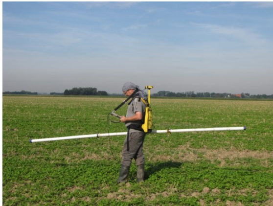
Figure 2.13: EM 31 instrument in an agricultural field.
