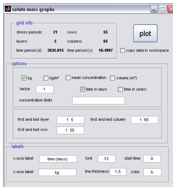
figure 4.15 GUI to calculate solute mass in a designated part of the aquifer.
