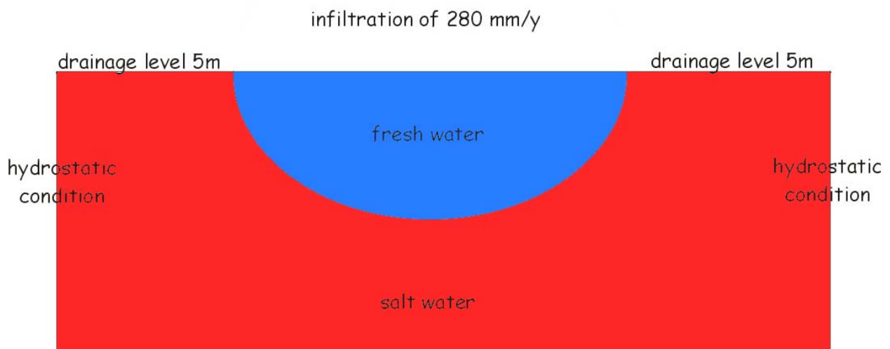
figure 6.23 Conceptual model for the formation of a fresh water lens in a coastal area.
