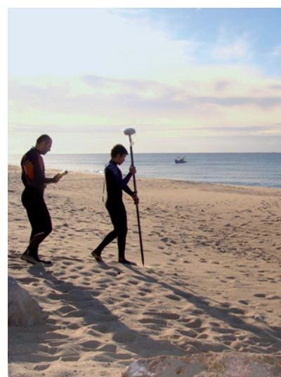
Three-dimensional beach surveying using GPS at Praia de Faro, Portugal.
