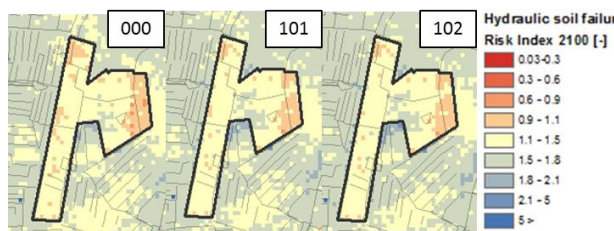
Figure 32 The hydraulic soil failure risk on land for the MT polder per scenario in 2100.
