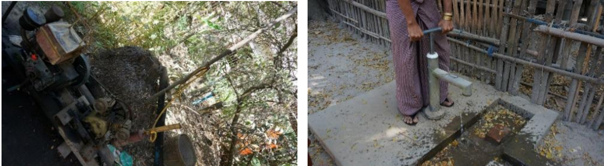
Figure 13a, b: automatically operated tube-well (a, left). The manual “Bangladeshi” well (b, right).
