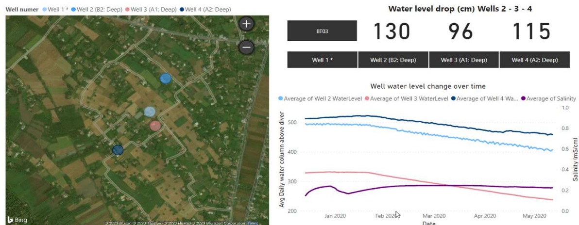
Figure 7. Map showing the location of the wells with installed divers (left). Graph showing the water level drop in cm in different wells from January to May (right) (Deltares, 2020).
