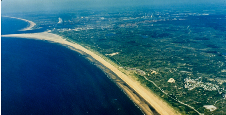
Fig. 6: Port of IJmuiden, sediment transport is directed in northern direction (i.e. towards the top left of the image). Accretion occurs at the south side of the breakwaters (source: RWS).
