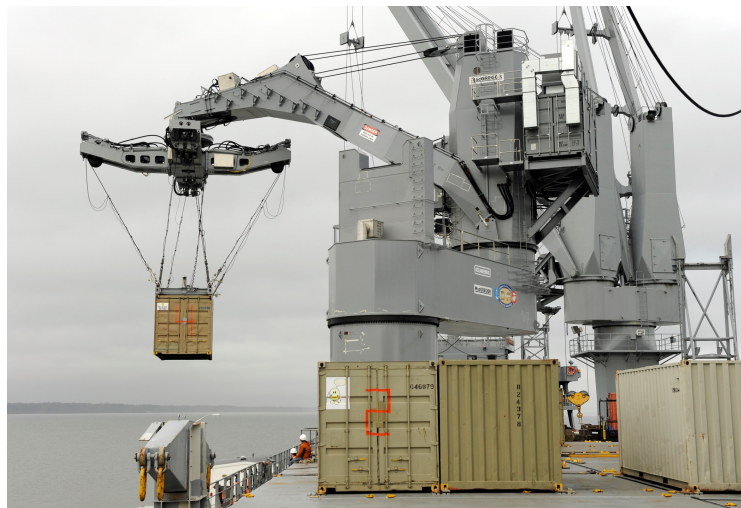
Fig. 4: The Large Vessel Interface Lift On/Lift Off (LVI Lo/Lo) Crane for ship-to-ship container transfer at sea (source: ONR, USA).
